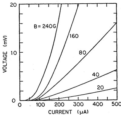
FIG. 1.  $I$ - $V$  characteristics for an aluminum film 200 Å thick with  $T_c = 1.7^\circ\text{K}$  taken at  $T = 1.33^\circ\text{K}$  for various values of perpendicular magnetic field. The normal resistance of the film was 435  $\Omega$ .  $H_{c2} = 300$  G.
