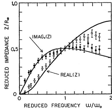
FIG. 2. Complex impedance versus frequency at  $T = 1.33^\circ\text{K}$  with a perpendicular magnetic field of 80 G. The solid lines are the real and imaginary parts of the impedance as given by Eq. (5); we have taken  $\omega_0/2\pi = 24$  Mc/sec and  $R_\infty = 38 \Omega$  to obtain the best fit.
