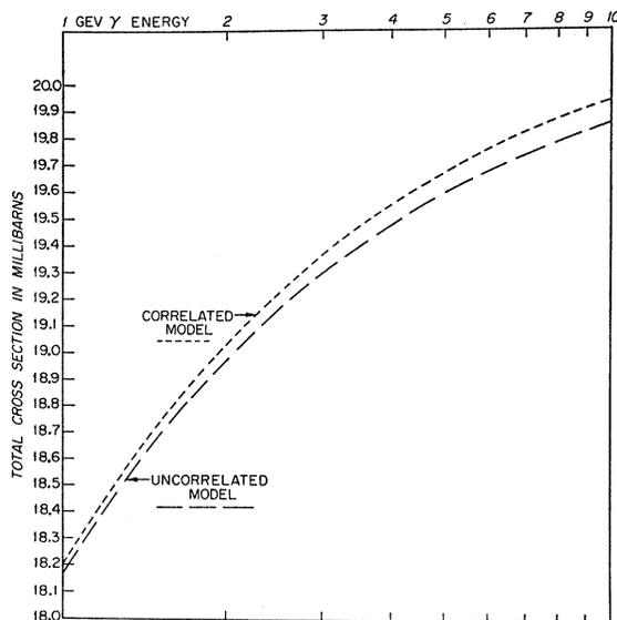
FIG. 2. Incoherent pair-production total cross section as in Fig. 1, for two different atomic models.
