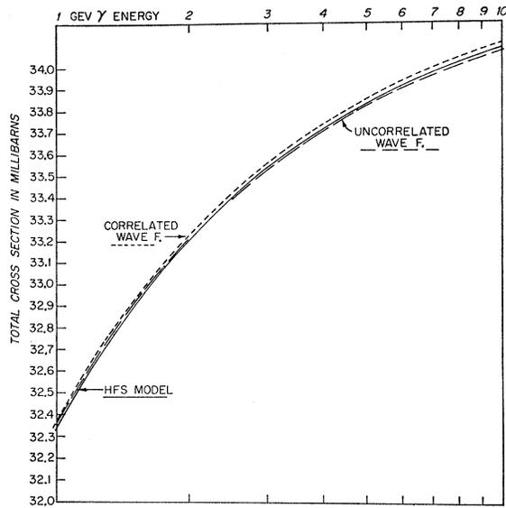
FIG. 1. Coherent pair-production total cross section versus the energy of the photon producing the pair, in helium, under the assumption of three different atomic models.
