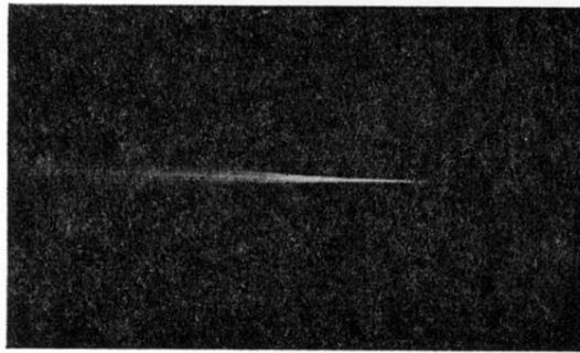
FIG. 14. Propagation of the focused laser beam in an 80% acetone, 20% carbon disulfide mixture. The laser light here is completely reflected by stimulated Brillouin scattering.
