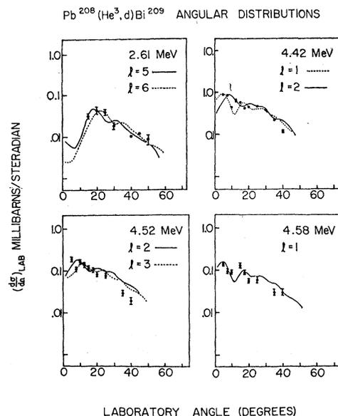
FIG. 3. Angular distributions of deuteron groups from Pb<sup>208</sup>(He<sup>3</sup>, d)Bi<sup>209</sup> at a He<sup>3</sup> energy of 44.2 MeV. The solid and dotted curves are the normalized reduced cross sections  $S_{ij}$  obtained from the DWA analysis.
