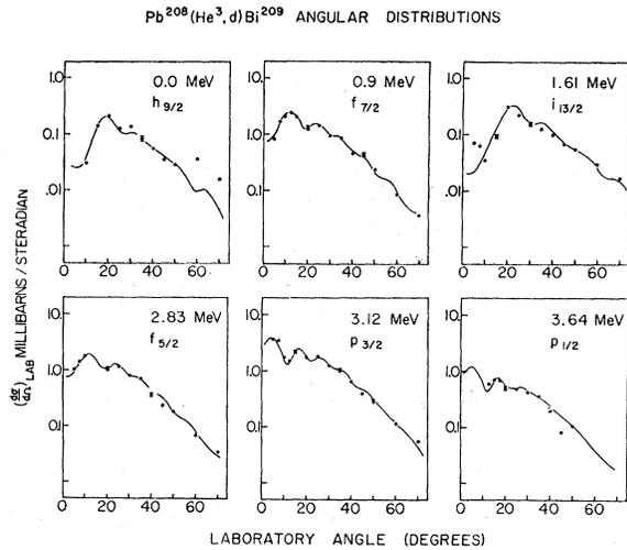
FIG. 2. Angular distributions of deuteron groups from Pb<sup>208</sup>(He<sup>3</sup>,d)Bi<sup>209</sup> at a He<sup>3</sup> energy of 44.2 MeV. The solid curves are the normalized reduced cross sections  $\sigma_{ij}$  obtained from the DWA analysis.
