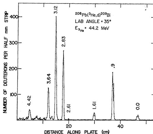
FIG. 1. Deuteron spectrum at 35° from the  $\text{Pb}^{208}(\text{He}^3, d)\text{Bi}^{209}$  reaction.
