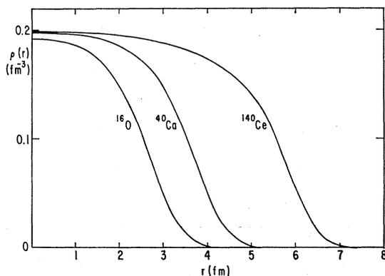
FIG. 5. Results for  $\text{O}^{16}$ ,  $\text{Ca}^{40}$ , and  $\text{Ce}^{140}$  obtained from the variational method for a modified Gaussian function with a cubic polynomial. Here  $\eta=5$ ,  $\xi=\frac{1}{5}$ .
