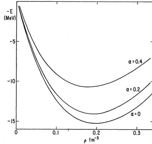
FIG. 1. Nuclear-matter saturation curves for various neutron excess. These are fitted to the results of Brueckner *et al.* (see Ref. 12).
