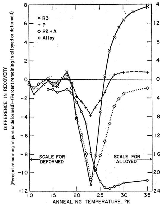
FIG. 4. The differences in recovery (the percentage of damage remaining in an untreated specimen minus the percentage remaining in specimens given various treatments before irradiation) versus the annealing temperature in stage I.
