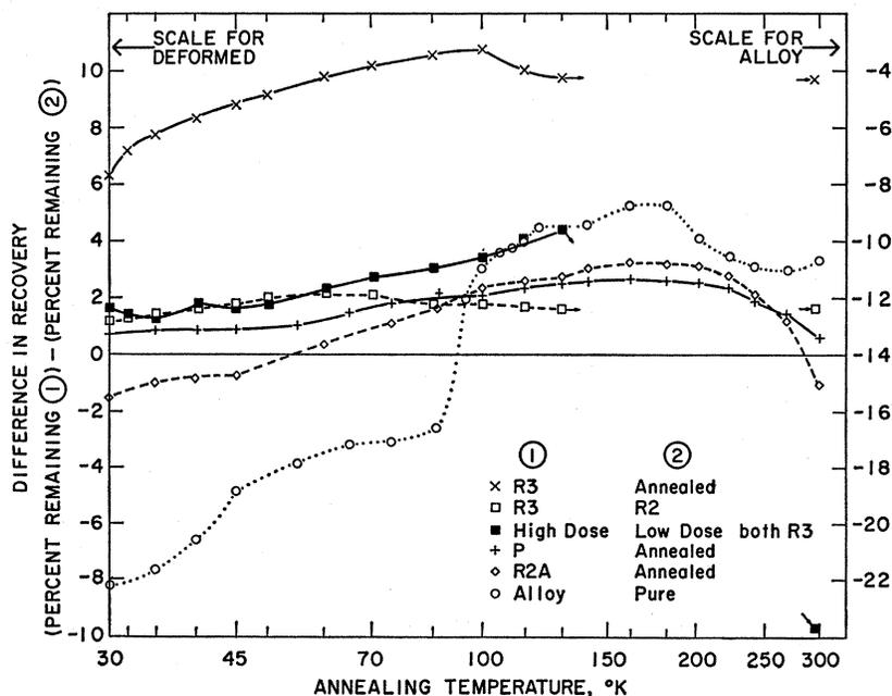
FIG. 8. The differences in percent recovery between pairs of specimens as a function of annealing temperature in stages II and III.
