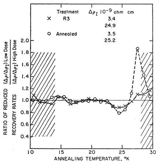
FIG. 6. The ratio of the normalized recovery rates  $[(\Delta R/\Delta T)/\Delta\rho_I]$  for two pairs of specimens given different doses.
