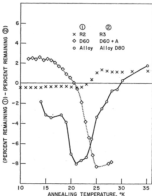
FIG. 5. The differences in recovery between specimens given various treatments before irradiation as a function of annealing temperature in stage I.
