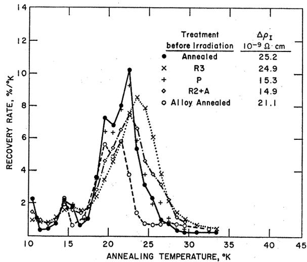
FIG. 3. The effect of various treatments on the stage-I recovery spectrum of Pt.
