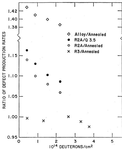
FIG. 1. The effect of various treatments on the initial defect production rates in Pt irradiated near 6°K with 20-MeV deuterons.
