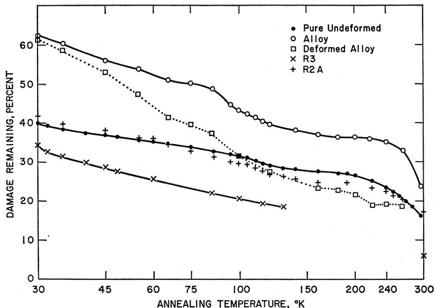
FIG. 7. Recovery in stages II and III of Pt given various treatments before irradiation with 20-MeV deuterons.
