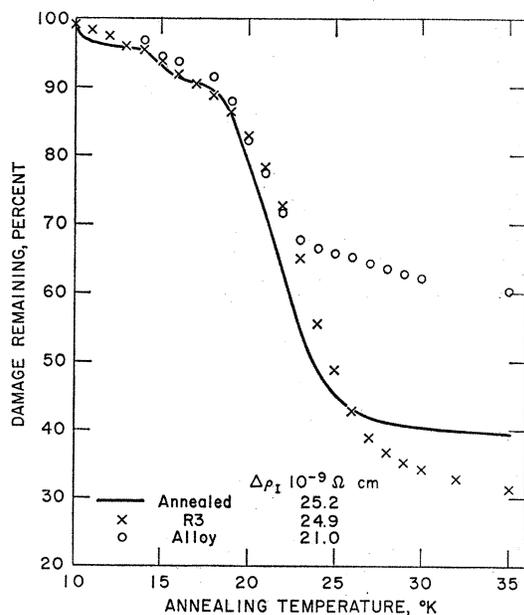
FIG. 2. The effect of deformation and of alloying with Au on stage-I recovery of dueteron-irradiated Pt.
