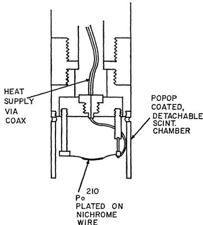
FIG. 1. The detachable scintillation chamber showing the  $\text{Po}^{210}$   $\alpha$  source on the heater wire.
