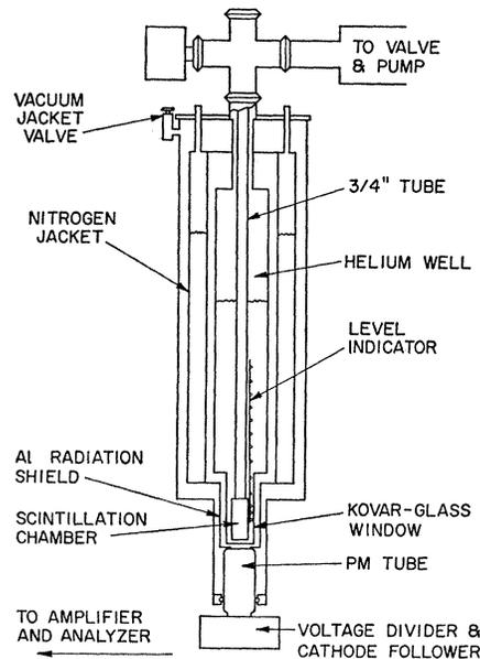
FIG. 2. Schematic drawing of the stainless steel Dewar used for scintillation measurements.
