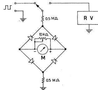
FIG. 2. Four-diode bridge comparator for the measurement of the square-wave voltage. RV: dc reference voltage, Keithley 241.
