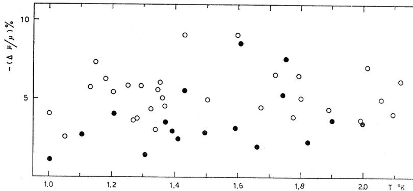
FIG. 10. The values of the relative size of the discontinuity  $\Delta\mu/\mu$  for the first step at various temperatures. The errors—discussed in the text—are of 50% and are not indicated for graphical clarity. Black points refer to negative ions, white points to positive ions.
