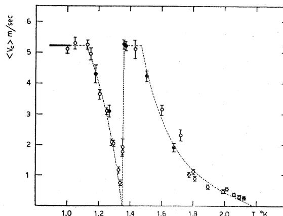
FIG. 7. Drift velocity of the first step for negative ions (upper curve) and for positive ions (lower curve) at various temperatures. The symbols are explained in the text. The dotted lines represent the functions (4)–(7) of the text.
