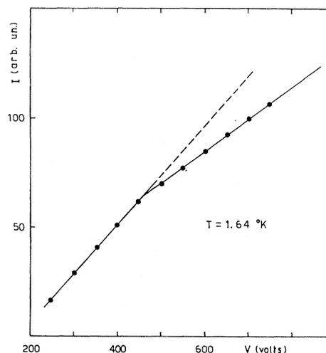
FIG. 4. Another example of the "square-wave current effect" which occurs at the critical voltage.
