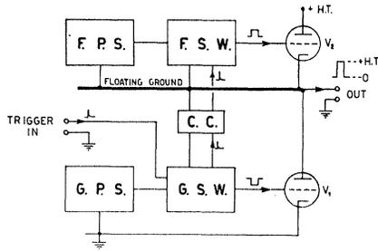
FIG. 1. Block diagram of the high-voltage square-wave generator used at high temperatures. GPS: grounded power supply. GSW: square-wave generator. FPS: floating power supply. FSW: floating square-wave generator. CC: coupling circuits between the grounded and the floating channels.
