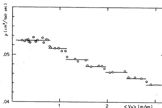
FIG. 6. An example of results with negative ions at  $2.00^\circ\text{K}$ , where steps up to the seventh have been detected. The first step is not present. If one takes for  $\langle v_1 \rangle$  the value of  $\frac{1}{2}\langle v_2 \rangle = 0.39$  m/sec, then for the other steps one has  $\langle v_n \rangle = n\langle v_1 \rangle$ , with  $n=3.0, 4.0, 5.0, 6.1, 7.1$ .
