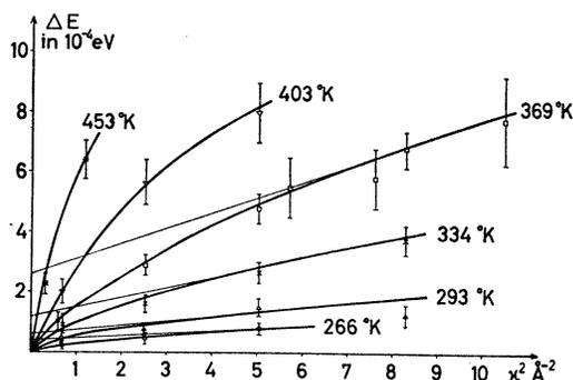
FIG. 3. Observed linewidth data on glycerol together with fitted theoretical linewidth forms given as solids lines. The best fit to the asymptotic behavior is shown for 266, 293, 334, and 369°K. The intercept on the  $\Delta E$  axis is  $2\hbar/\tau_{00}$ . The slope of the asymptote is  $2\hbar D_p$ .
