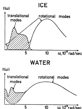
FIG. 10. Observed shapes of the frequency distributions in ice and water and the proposed division into a hindered translational and a hindered rotational component.
