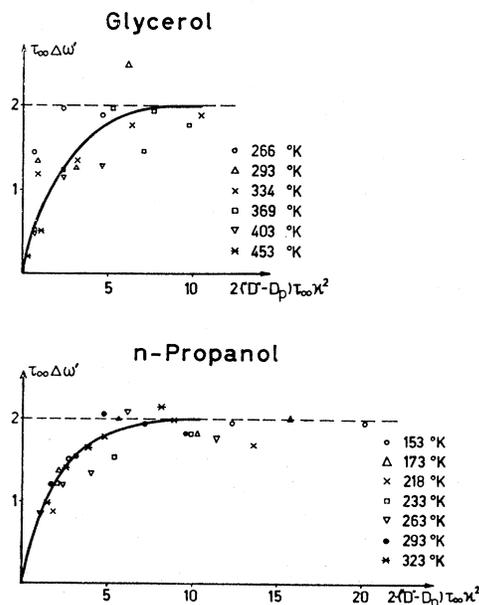
FIG. 7. The generalized plot of linewidth data obtained from quasi-elastic neutron scattering in glycerol and *n*-propanol. The solid line represents the calculated average linewidth curve.
