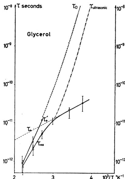
FIG. 4. Relaxation times  $\tau_{00}$ ,  $\tau_0$ , and  $\tau_0'$  for glycerol derived from the neutron data. The observed dielectric and ultrasonic relaxation times are shown as dashed and dash-dot lines, respectively. Part of the dielectric data are extrapolated by use of a formula proposed by McDuffie and Litowitz.
