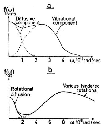
FIG. 8. Possible shapes of the frequency distribution for (a) hindered translations corresponding to the center-of-gravity motion and (b) hindered rotations corresponding to motions relative to the center of gravity.
