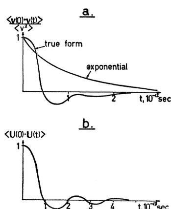
FIG. 9. Possible shapes for the self-correlation functions which form the basis for the frequency distributions of Fig. 8: (a) the velocity autocorrelation function corresponding to the center-of-gravity motion, (b) the angular autocorrelation function corresponding to the relative, hindered rotational motion.
