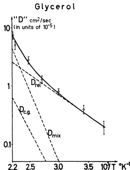
FIG. 5. Observed diffusion coefficient " $D$ ". The various theoretical components  $D$ ,  $D_{mix}$ , and  $D_{rel}$  are shown as dashed lines. The full line is the sum of these components.
