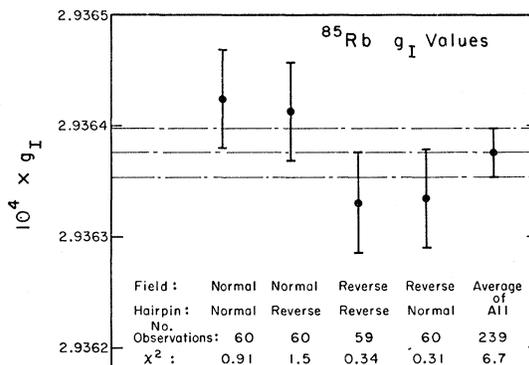
FIG. 3. The results of the least-squares analysis of our data, assuming  $g_J(^{85}\text{Rb}) = -2.0023319$ . The indicated errors represent one standard deviation.
