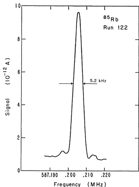
FIG. 2. A  $^{85}\text{Rb}$   $(3, -1) \leftrightarrow (3, -2)$  resonance obtained at 2076 G.
