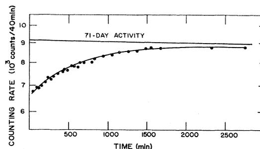
FIG. 2. Count rate for the 0.81-MeV  $\gamma$  line from  $^{58}\text{Co}$  produced by the  $(\gamma, np)$  reaction. Irradiation time 210 min. End of irradiation at  $t=0$ . Semilogarithmic plot.
