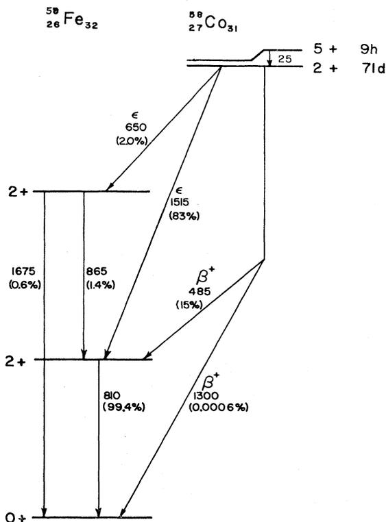
FIG. 1. Decay scheme of  $^{58}\text{Co}$ . Energies in keV.
