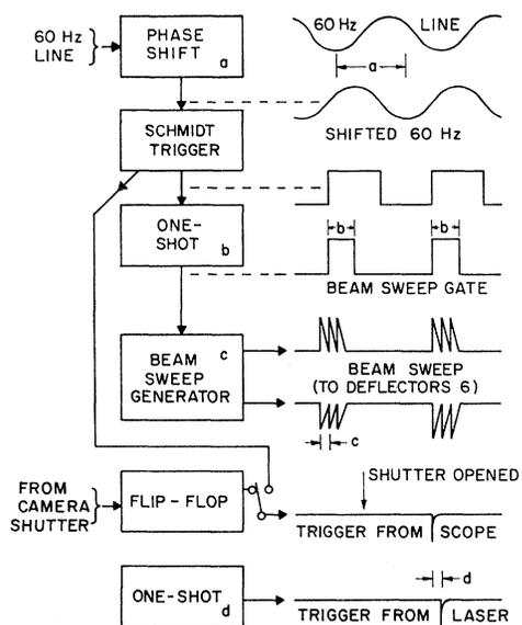
FIG. 2. Timing circuits. Letters a-d indicate variable timing adjustments and the circuits in which they are made: (a) 60-Hz phase adjustment; (b) beam sweep on-time; (c) beam sweep period; (d) laser trigger delay.
