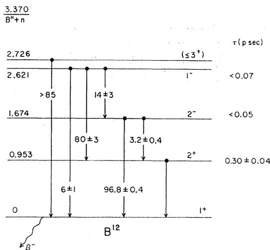
FIG. 3. Level diagram for the bound levels of  $B^{12}$ , summarizing the excitation energies and branching ratios determined in this and previous reports, as cited in the text. Values or limits determined for the mean lifetimes of these states are indicated also; the various references are cited in Sec. V of the text.
