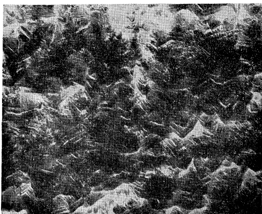
FIG. 4. Electron micrograph of a calcium fluoride film. Note that detail of the order of 0.01 \mu ( 100 \text{ \AA} ) can be seen.
