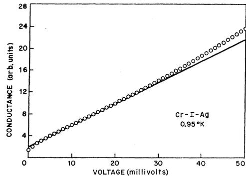
FIG. 18. Conductance versus voltage at 0.95°K for the Cr-I-Ag junction of Fig. 17.
