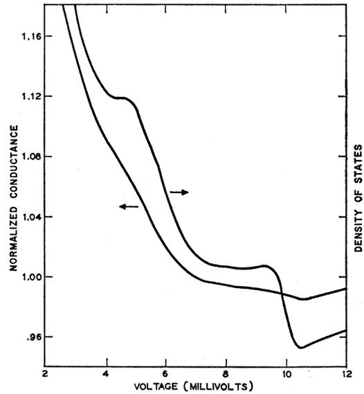
FIG. 20. The normalized derivative of a Cr- $I$ -Pb junction at  $0.9^\circ\text{K}$  compared with the density of states calculated from measurements of a Pb- $I$ -Pb junction at  $0.9^\circ\text{K}$ .
