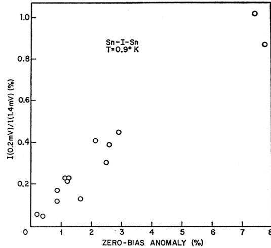
FIG. 14. A plot of superconducting background (defined in the text) versus the magnitude of the zero-bias anomaly.
