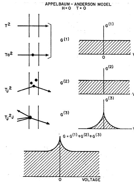
FIG. 2. Schematic drawings of the different processes that contribute to the theoretical conductance of the Appelbaum model. The magnetic impurities are represented by black dots inside the insulating barriers. The scattering of the tunneling electrons is represented by arrows on the left, the resulting conductances are shown on the right, and the total conductance is at the bottom.
