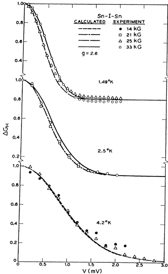
FIG. 8. Comparison between experimental and theoretical voltage dependences of  $\Delta G_H$  at different temperatures and fields. The only unknown parameter used here is the value of  $g$ .
