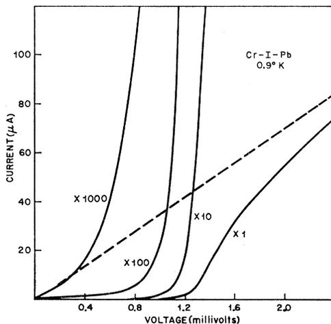
FIG. 19. Current versus voltage for a Cr- $I$ -Pb junction at  $0.9^\circ\text{K}$  with no applied magnetic field. The dashed line is the characteristic with Pb in the normal state. The current scales have been expanded by decades as shown.
