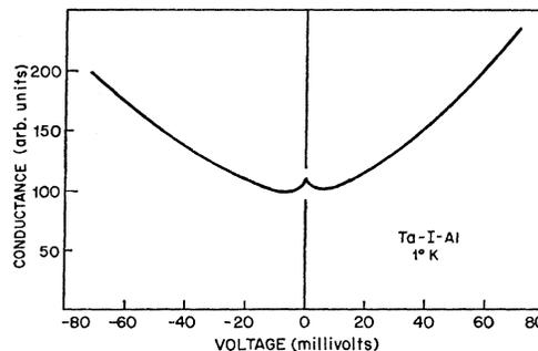
FIG. 1. Dynamic conductance versus voltage for a Ta-I-Al junction at 1°K. A field of 3 kG was used to keep the tantalum normal.
