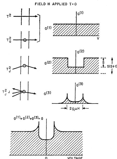
FIG. 5. Schematic drawings of the same processes of Fig. 2 under the influence of an external field. A Zeeman splitting is produced on the impurity spins which are represented by open circles on the left. The corresponding conductances are shown on the right. The total conductance is shown on the bottom.
