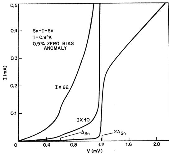
FIG. 13. I-V characteristics for a typical Sn-Sn junction. The position of  $\Delta_{Sn}$  is marked on the diagram. The current scales have been expanded as shown.
