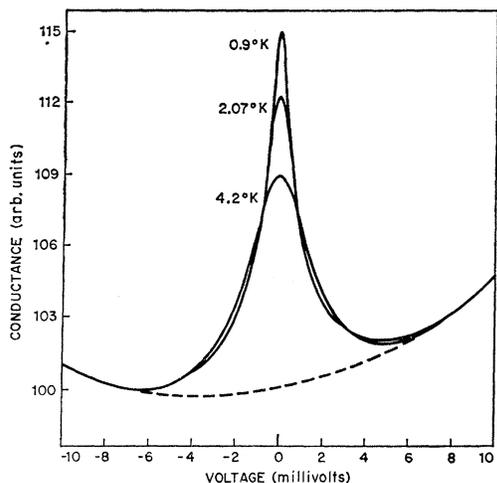
FIG. 3. The temperature dependence of a Ta-I-Al junction as shown on a  $G$ -versus- $V$  plot. The applied magnetic field is 3 kG.
