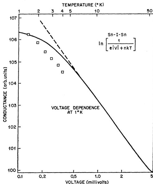
FIG. 4. The temperature dependence of  $G^{(3)}(0)$  and the voltage dependence of  $G^{(3)}(V)$  at 1°K for a Sn-I-Sn junction.  $G(0)$  is plotted against  $\ln T$  on the upper abscissa, and  $G(V)$  is plotted against  $\ln V$  on the lower abscissa. The value of  $eV$  is made equal to  $kT$  on this plot. A similar plot is obtained for Ta-I-Al junctions.
