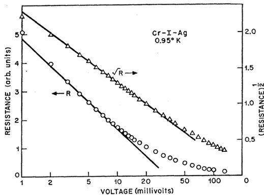
FIG. 17. Resistance and  $(\text{resistance})^{1/2}$  versus  $\ln V$  at 0.95°K for a Cr-I-Ag junction.
