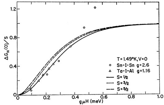
FIG. 10. The changes in  $\Delta G_H(0)$  from Fig. 9 are normalized with respect to the spin value and comparison made between theory and experiment for Sn-I-Sn and Ta-I-Al junctions at 1.49°K.
