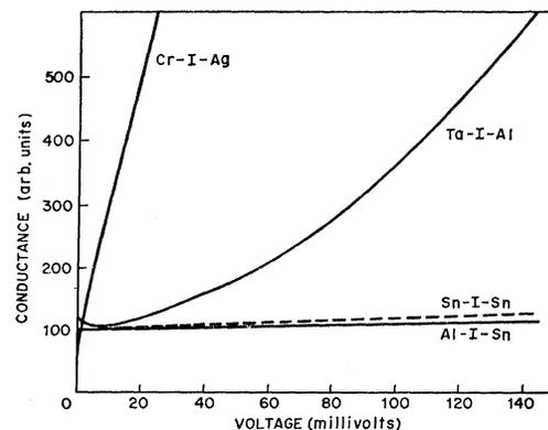
FIG. 12. Conductances versus voltage plot of several normal metal junctions which exhibit different zero-bias behaviors. The temperature is 1°K.
