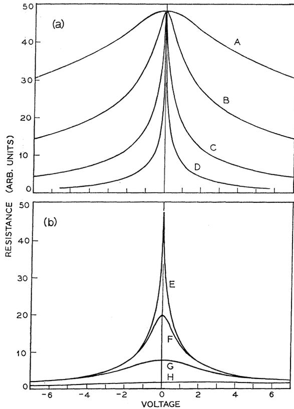
FIG. 16. (a) The dynamic resistance versus voltage for a Cr-I-Ag junction at 0.9°K. The voltage scales are A=0.2 mV/div, B=1.0 mV/div, C=5 mV/div, D=20 mV/division. (b) The dynamic resistance versus voltage for a Cr-I-Ag junction at various temperatures, E=0.9, F=20.4, G=77, and H=290°K. The voltage scale is 10 mV/division.
