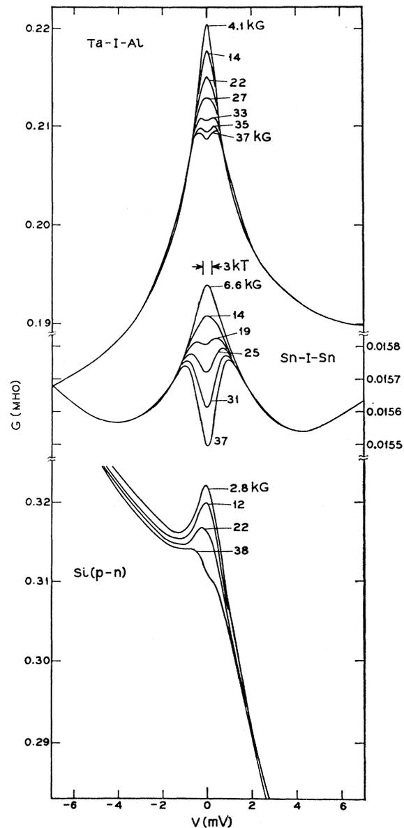
Fig. 6. Conductance-versus-voltage plots for Ta-I-Al (upper trace), Sn-I-Sn and silicon *p-n* junctions (lower trace) at 1.5°K. The magnitudes of the applied magnetic fields are indicated. Above the Sn-I-Sn trace the voltage corresponding to  $3kT$  is shown.
