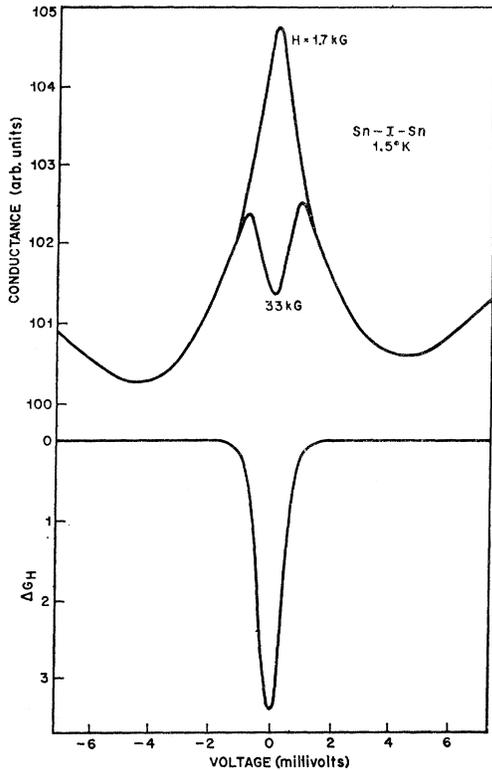
FIG. 7. Conductance-versus-voltage plot for a Sn-I-Sn junction (upper trace) in two fields (1.7 and 33 kG) and the differences  $\Delta G_H$  between the two curves (lower trace).
