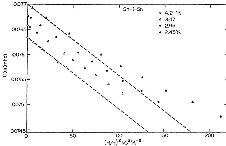
FIG. 11. Conductance measured at zero bias versus  $H^2/T^2$  plot at different temperature for a Sn-I-Sn junction. The two dashed lines are parallel.
