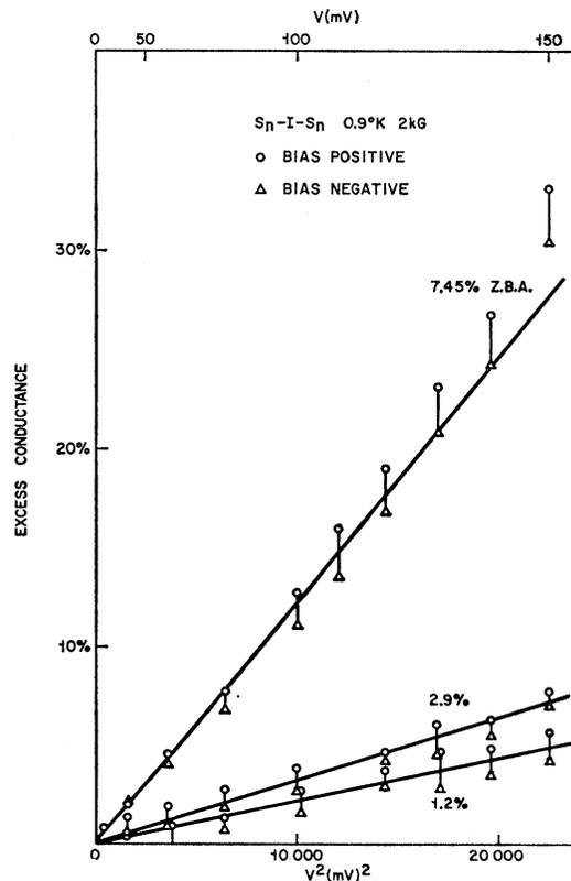
FIG. 15. Excess conductance above the lowest background junction (0.2% zero-bias anomaly) plotted versus  $V^2$  for two directions of bias. The polarity refers to the tin film on which the oxide is grown.
