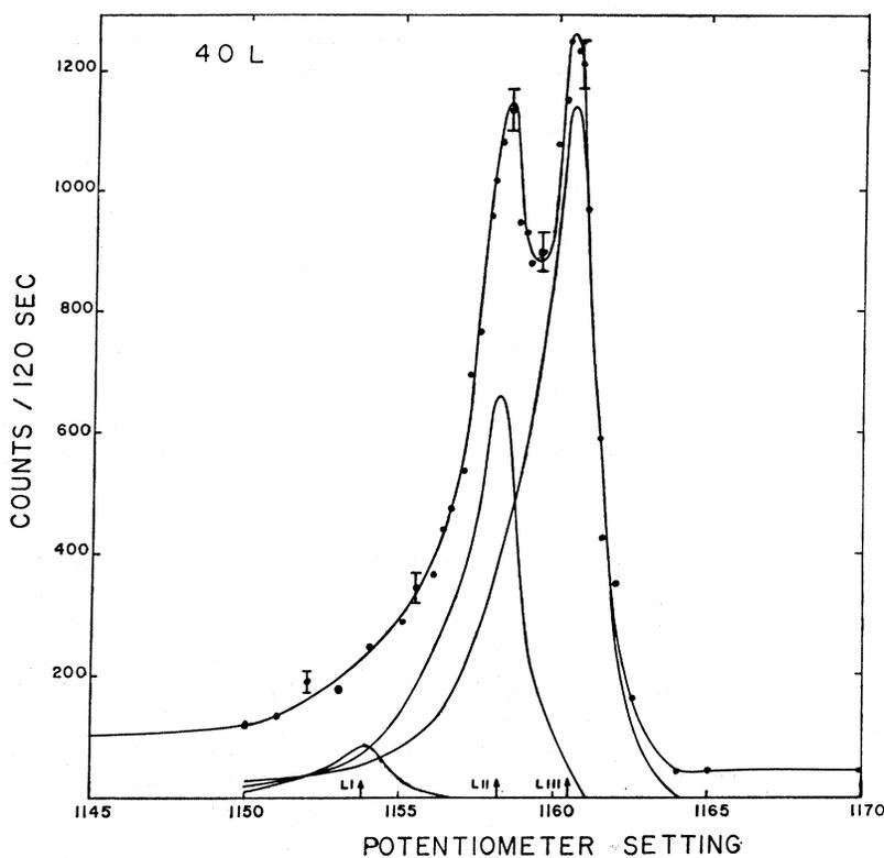
FIG. 2. 40L line for the isomeric transition in  $\text{Rh}^{103}$ . Experimental momentum resolution (including source thickness effects) is 0.19%. Also shown are the three  $L$ -subshell lines (solid curves) and the composite  $L$  line (solid curve through the data points). The solid curves were obtained by least-square techniques with  $\chi^2=1.72$  and  $|\delta|=0.08$  for  $M4/E3$  mixing. Conversion coefficients of Sliv and Band (see Ref. 18) were used in this calculation.
