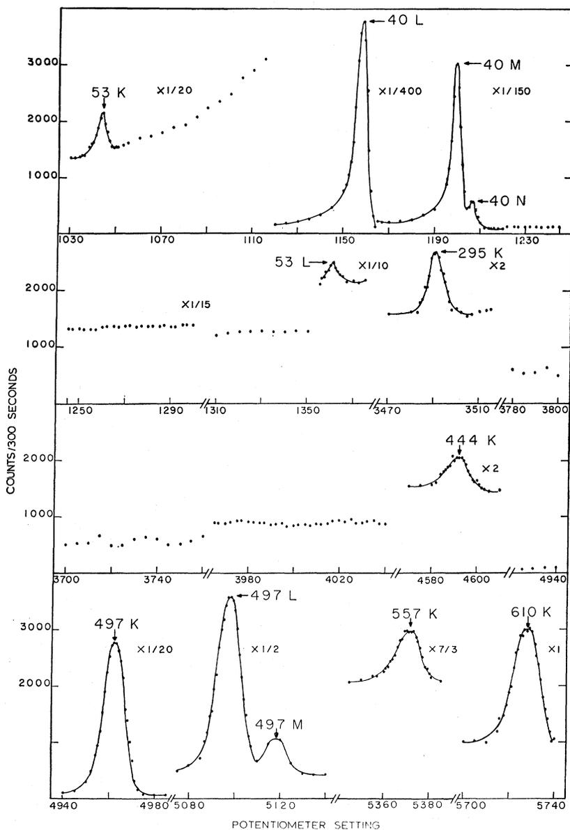
FIG. 1. Partial internal-conversion-electron spectrum showing the major observed lines and regions of the spectrum where the 67K, 322K, and 362K lines are expected.
