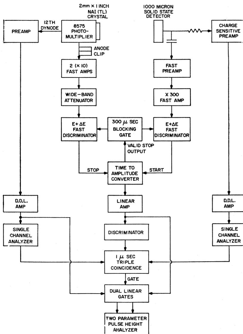
Fig. 1. Block diagram of electronics.
