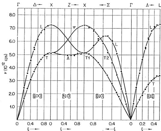
FIG. 3. The phonon dispersion curves for copper in the major symmetry directions at 49°K. The lines shown represent the sixth-nearest-neighbor AS force model.
