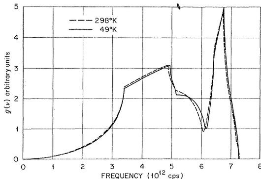
FIG. 4. Frequency distributions at 49 and 298°K for copper.
