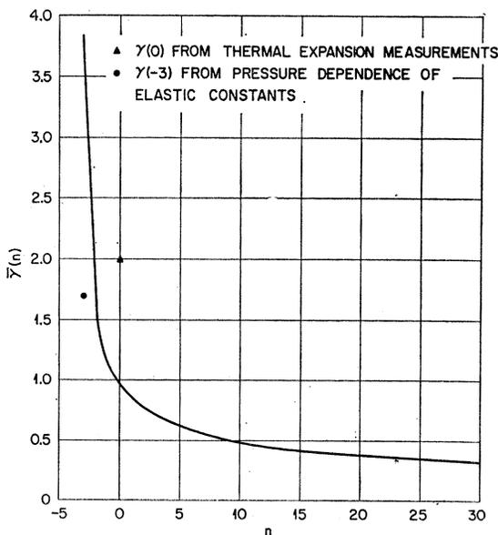
FIG. 6. The  $\bar{\gamma}(n)$  obtained from the variation of  $\nu_n$  with temperature using Eq. (6).  $\gamma(0)$  and  $\gamma(-3)$  were taken from Ref. 19.
