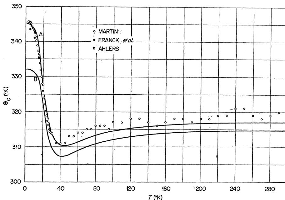
FIG. 7. Comparison of the calculated  $\Theta_c(T)$  with experiment. Curves A and B were calculated with  $g(\nu)$  at 49 and 298°K, respectively. The experimental results were obtained from Refs. 16, 17, and 22.
