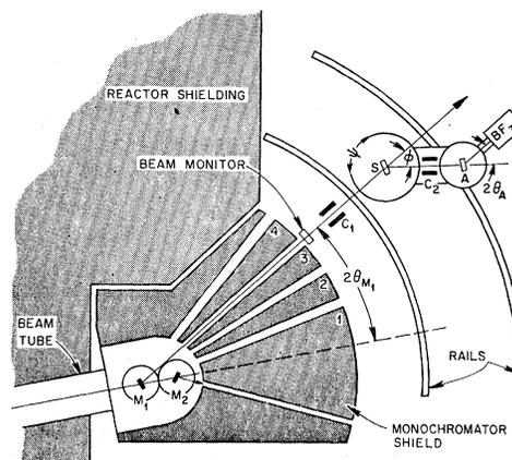
Schematic For Triple-axis Neutron Spectrometer at ORR
