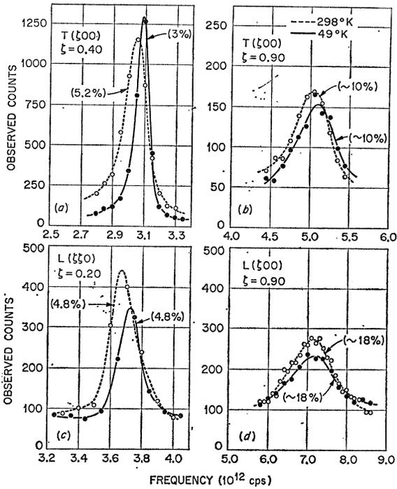
FIG. 2. Several typical phonon peaks for copper obtained in constant-*Q* experiments.
