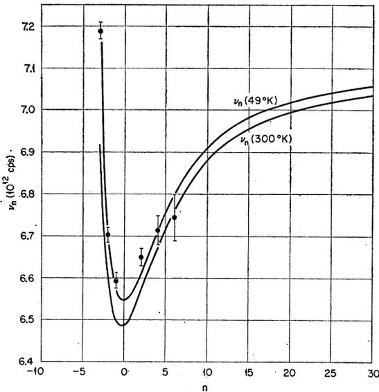
FIG. 5. Debye "cutoff" frequencies  $\nu_n$  obtained from  $g(\nu)$  at 49 and 298°K. The experimental points were taken from Salter (Ref. 15).
