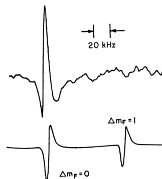
FIG. 9. The upper trace is the output of the 462-MHz light-beat detection system. An asymmetric line shape is shown. The lower trace is the output of the zero-frequency detection system.
