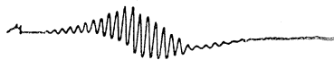
FIG. 2. The hyperfine structure on the \frac{1}{2} \rightarrow -\frac{1}{2} transition of \text{Fe}^{3+} in \text{KTaO}_3 caused by the nuclear spins of the \text{K}^{+1} ions.
