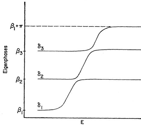
FIG. 2. Eigenphases for a typical 3-channel resonance, showing two eigenphase repulsions; constant backgrounds have been assumed for clarity. Note that as the resonance energy is passed,  $\delta_1$  rises from  $\beta_1$  to  $\beta_2$ ,  $\delta_2$  rises from  $\beta_2$  to  $\beta_3$ , and  $\delta_3$  rises from  $\beta_3$  to  $\beta_1 \pmod{\pi}$ .
