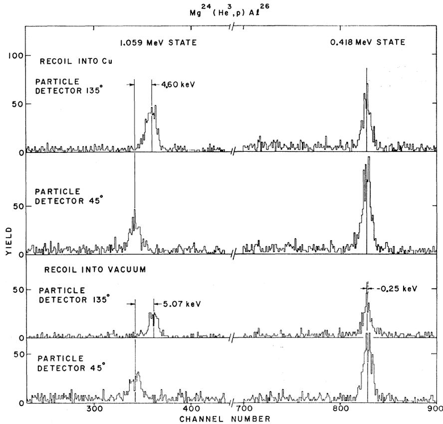
FIG. 3. Spectra showing the Doppler shifts for the 830- and 418-keV  $\gamma$  rays from the  $Mg^{24}(He^3,p)Al^{26}$  reaction when the recoils were stopped in nickel and when they were allowed out into the vacuum.
