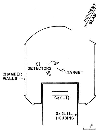
FIG. 2. Schematic diagram of the experimental arrangement used for the Doppler-shift measurements.
