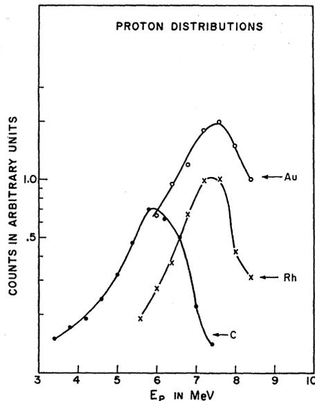
FIG. 4. Typical proton energy distributions for Au, Rh, and C for neutron angle of  $-20^\circ$  and proton angle of  $-50^\circ$ . The incident deuteron energy is 12 MeV.
