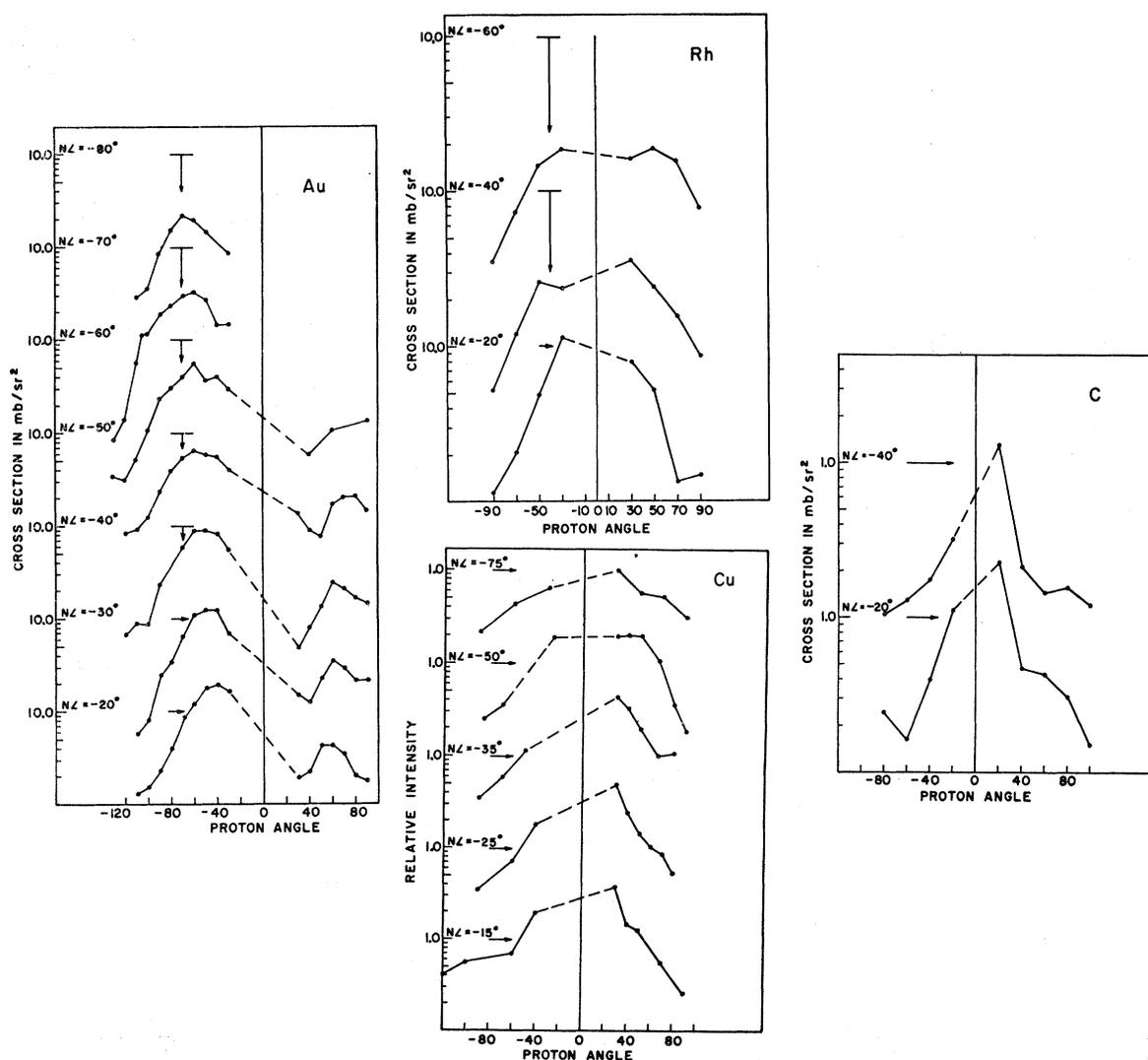
FIG. 2. Proton angular distributions for Au, Rh, Cu, and C at 12-MeV for various neutron angles. Negative proton angles correspond to the neutron and proton detector in the same side of the incident beam. The beam direction is designated by a vertical line at  $0^\circ$ . The scale on the ordinate to be used for each curve is indicated with an arrow. The neutron angle for each curve is also indicated by the arrow.
