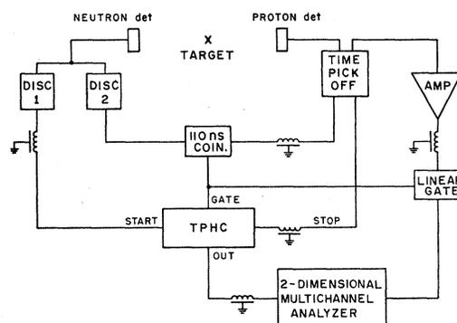
FIG. 1. Electronic setup for the deuteron-disintegration experiment. Various delays for correct signal timing in the proton and neutron legs are indicated schematically.
