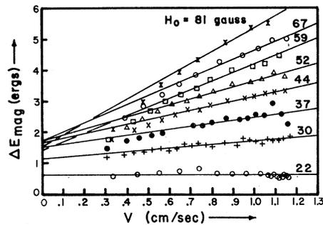
FIG. 4. Energy dissipation per swing as a function of speed for the 0.0508-cm strips at 3°K for various field strengths.
