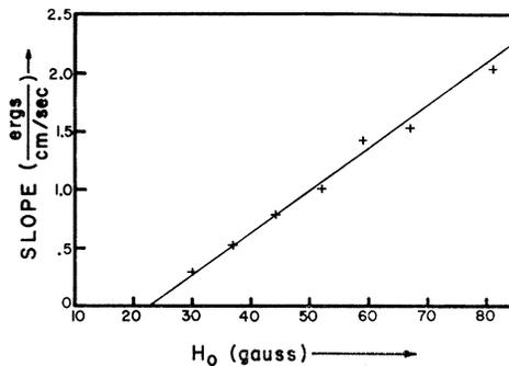
FIG. 5. Slopes of the energy dissipation-speed curves as a function of the field strength for the 0.0508-cm strips at 3°K.
