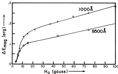
FIG. 3. Energy dissipation per swing as a function of the localized field strength for the 1000 and the 8000 Å films. The difference between the curves is attributed to the relative qualities of the films.
