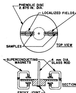
FIG. 1. Sketch of the arrangement of the torsion pendulum and the magnets in the equilibrium position.
