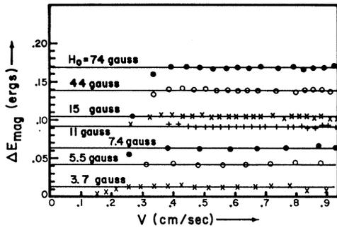
FIG. 2. Energy dissipation per swing as a function of the speed with which the 8500 Å films at 3°K passed through the field. The energy dissipation is independent of the speed but increases with the field intensity.
