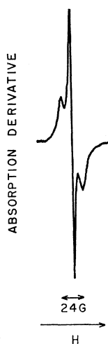
FIG. 3. High-field member of the set of six lines comprising spectrum III, which has nearly the same A as CaO:Mn 2+ . Separation of the outer peaks, 24 G. Room temperature; there is no angular dependence.
