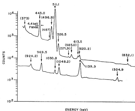
FIG. 2. Spectrum of low-energy  $\gamma$  rays from  $^{128}\text{Ba}$ - $^{128}\text{Cs}$ , observed with 8-cc Ge(Li) detector. Energies of  $\gamma$  rays from the  $^{131}\text{Ba}$  contaminant are given in parentheses.
