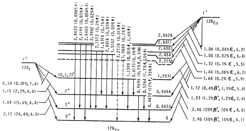
FIG. 6. Level scheme of  $^{128}\text{Xe}$ . Energies are quoted in MeV.  $\gamma$ -ray intensities, expressed in terms of percent of decays of the  $^{128}\text{I}$  ( $\leftarrow$ ) or  $^{128}\text{Cs}$  ( $\rightarrow$ ) parent isotope, are given in parentheses.
