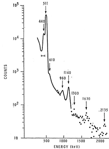
FIG. 4. Spectrum of  $\gamma$  rays in coincidence with the 443.2-keV  $\gamma$  ray of  $^{128}\text{Cs}$ , observed with NaI(Tl) detector.
