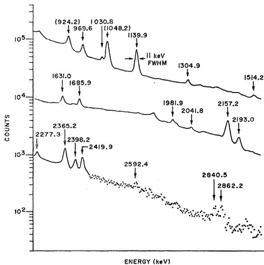
FIG. 3. Spectrum of high-energy  $\gamma$  rays from  $^{128}\text{Ba}$ - $^{128}\text{Cs}$ , observed with 30-cc Ge(Li) detector. Energies of  $\gamma$  rays from the  $^{131}\text{Ba}$  contaminant are given in parentheses.
