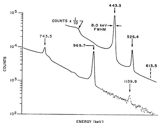
FIG. 1. Spectrum of  $\gamma$  rays from  $^{128}\text{I}$ , observed with 30-cc Ge(Li) detector.
