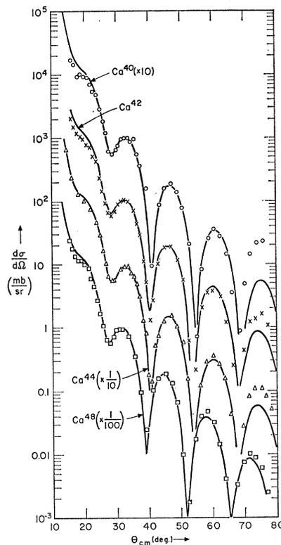
FIG. 2. Elastic scattering cross sections for 31-MeV  $\alpha$  particles from Ca<sup>40,42,44,48</sup>. The solid lines are optical-model fits to the data. The parameters for these fits are given in Table II.
