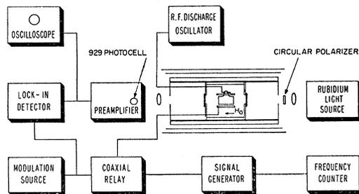
FIG. 3. A block diagram of the optical-pumping apparatus.
