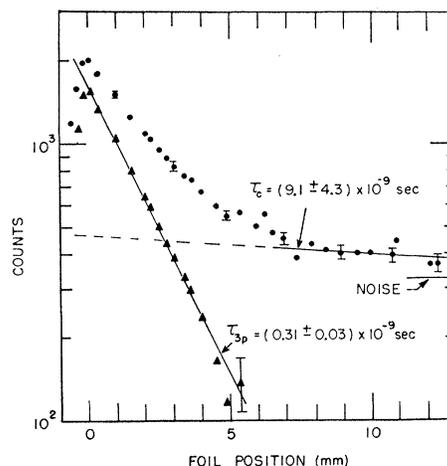
FIG. 2. Counts versus foil position for the line He II 256 Å. The counting interval for each point was 100 sec, the foil thickness was 500 Å, and the beam energy was 1 MeV. ●, uncorrected data; ▲, data corrected for both background and cascading.
