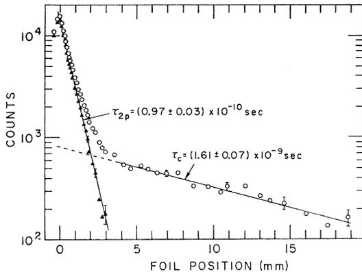
FIG. 1. Counts versus foil position for the line He II 304 Å. The data were obtained with a foil thickness of 500 Å, a beam energy of 1 MeV, and a counting interval of 100 sec. O, data corrected for background; ▲, data corrected for both noise and cascading.
