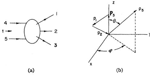
FIG. 4. (a) Production process  $4+5 \rightarrow 1+2+3$ . (b) Coordinate system for process (4a).
