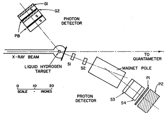
FIG. 1. Experimental arrangement.
