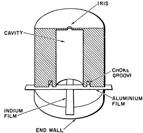
FIG. 1. A sectional view of the microwave cavity showing tunneling junction in position against the end wall. The superconducting strips are insulated from the cavity.
