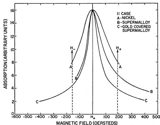
FIG. 1. Absorption with magnetic field parallel to surface of sample.
