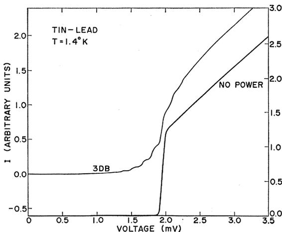
FIG. 6. Current-versus-voltage plots for the junction of Fig. 5 with a higher value of microwave power. The zero-power result has been included with the zero shifted for reference purposes.
