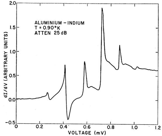
FIG. 4. Conductance versus voltage for the junction of Fig. 3 with 25 dB relative attenuation. This corresponds to a microwave power of approximately  $2\mu\text{W}$  dissipated in the cavity.
