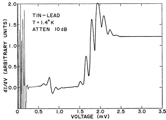
FIG. 5. Conductance versus voltage for a Sn-Pb junction. The power for this curve was chosen to demonstrate the additional multiphoton process associated with the peak at (a) and (b), as discussed in the text.
