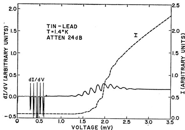
FIG. 8. Conductance and current for a Sn-Pb junction with films thinner than those of Figs. 5 and 6, showing increased interaction. Note that the structure in the conductance around 0.5 mV is due to the microwave Josephson-current interaction.
