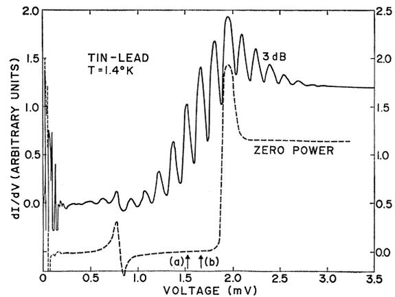
FIG. 7. Conductance versus voltage for the junction and conditions of Fig. 6. The arrows (b) and (a) indicate the position of the peaks  $N=2$  and  $N=3$ , respectively, occurring below the tunneling edge for which the detailed comparison with theory has been made.
