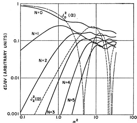
FIG. 11. Relative conductance as a function of relative microwave power shown by solid lines, and  $J_n^2$  shown in broken lines. The index  $N$  refers to the order of the multiphoton process.
