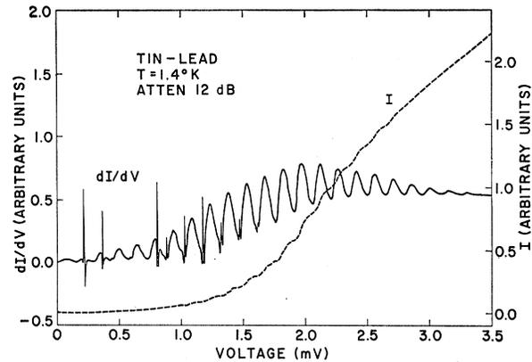
FIG. 9. Conductance and current for the diode of Fig. 7, showing the saturation of peak heights at increased power. In this plot the gain is 2.5 greater than that of Fig. 8.
