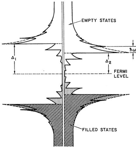
FIG. 10. Modified density-of-states function shown by solid lines, and the density-of-states function at zero power shown by dashed lines.
