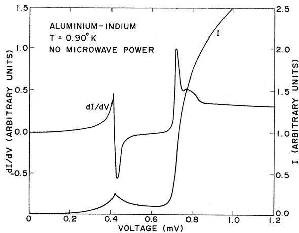
FIG. 3. Current  $I$  and conductance  $dI/dV$  versus voltage for an Al-In junction at  $0.9^\circ\text{K}$ . The zeros of  $I$  and  $dI/dV$  have been displaced for clarity.
