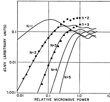
FIG. 12. Computed relative conductance versus relative microwave power for  $N=0, 1, 2, 3, 4$ , and  $5$ , with experimental points for  $N=2$  and  $3$  from the peaks indicated by arrows [(a) and (b)] in Fig. 7.
