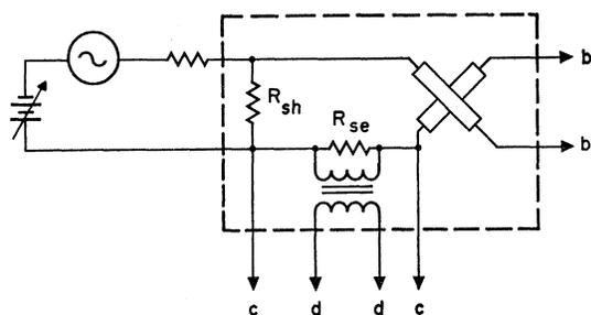
FIG. 2. Simplified diagram of the measuring circuit. Components inside the dotted box are within the Dewar. Conductance is computed from the voltage between the leads (d, d).
