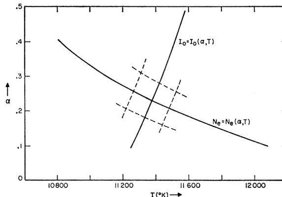
FIG. 3. Graphical solution for temperature  $T$  and sulfur-oxygen density ratio  $\alpha$  for radial position of 0.4 mm. Dotted lines represent estimated uncertainties in the positions of the curves.
