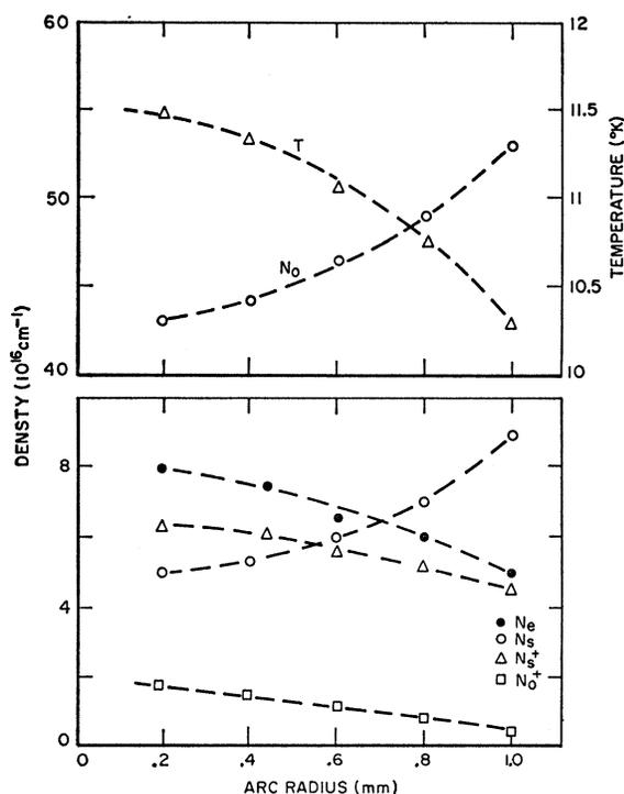
FIG. 4. Radial distribution of the various densities and the temperature in the arc. (The subscripts at the densities  $N$  denote: S=neutral sulfur, S<sup>+</sup>=singly ionized sulfur, O=neutral oxygen, O<sup>+</sup>=singly ionized oxygen,  $e$ =electrons).
