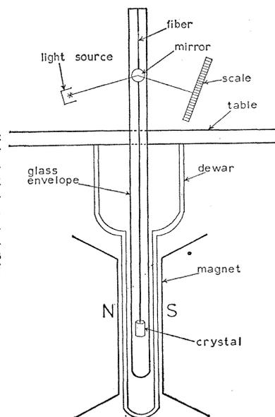
FIG. 1. Schematic drawing of the very sensitive magnetometer and cryostat used for the magnetic measurements. One mm deflection of the light beam on the scale arises from a torque of  $1.5 \times 10^{-4}$  dyn cm.
