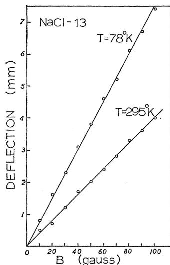
FIG. 2. Torque versus applied magnetic field for NaCl-13 at two different temperatures, 78°K and 295°K.
