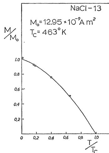
FIG. 3. The temperature dependence of the permanent magnetic moment for NaCl-13. The theoretical curve for spin waves in a ferromagnet is made to pass through the observed points in order to deduce a Curie temperature of 463°K.  $M = M_0[1 - (T/T_c)^{3/2}]$ .
