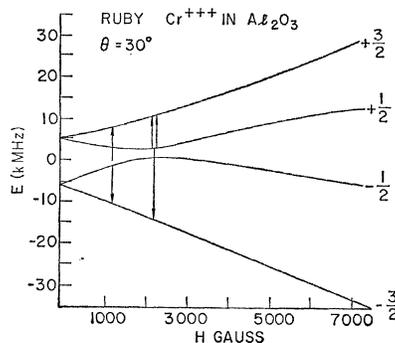
FIG. 1. Ruby ground-state Zeeman levels and cross-relaxation transitions.
