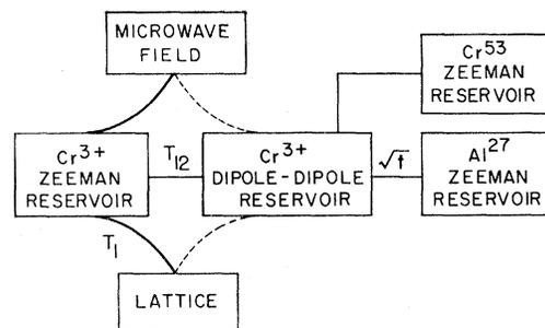
FIG. 6. Electron and nuclear spin-coupling scheme in dilute ruby.
