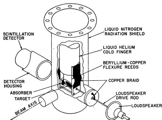
FIG. 2. Schematic diagram of the cryogenic target chamber employed in Mössbauer experiments following Coulomb excitation.
