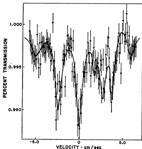
FIG. 11. Mössbauer absorption spectrum following Coulomb excitation of the 73.4-keV state of  $Dy^{164}$  at 4.2°K for a  $Dy_2O_3$  absorber containing 20 mg/cm<sup>2</sup> of  $Dy^{164}$ . These data have been corrected for nonresonant background.
