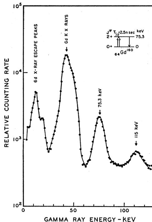
FIG. 7. Gamma-ray spectrum following Coulomb excitation of  $Gd_2^{160}O_3$ .
