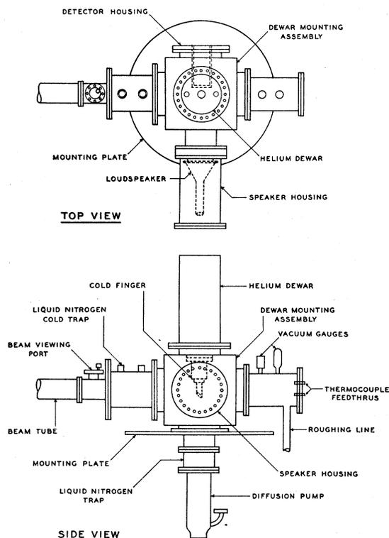
FIG. 3. Schematic diagram of the details of the helium cold finger and Mössbauer absorber assembly.
