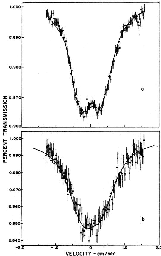
FIG. 9. Mössbauer absorption spectra following Coulomb excitation of the 75.3-keV state of  $Gd^{160}$  at 4.2°K for (a)  $GdAl_2$  absorber containing 21 mg/cm<sup>2</sup> of  $Gd^{160}$  and (b) metallic Gd absorber containing 46 mg/cm<sup>2</sup> of  $Gd^{160}$ . These data have been corrected for nonresonant background.
