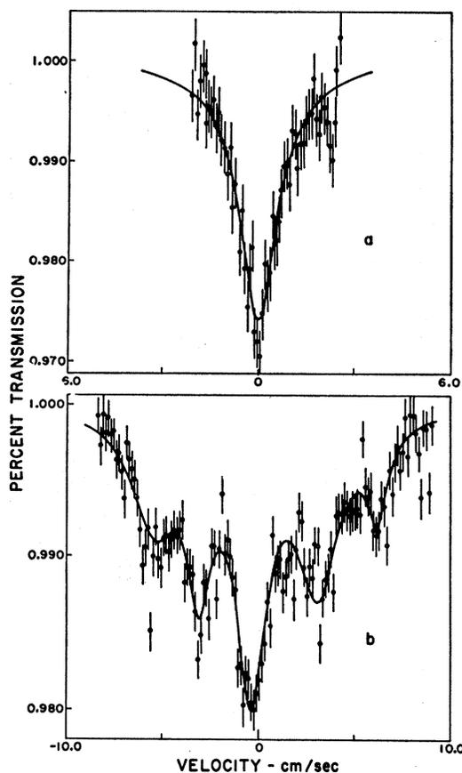
FIG. 12. Mössbauer absorption spectra following Coulomb excitation of the 79.8-keV state of  $Er^{168}$  at 4.2°K for (a)  $Er_2O_3$  absorber containing 62 mg/cm<sup>2</sup> of  $Er^{168}$  and (b) metallic erbium absorber containing 31 mg/cm of  $Er^{168}$ . These data have been corrected for nonresonant background.
