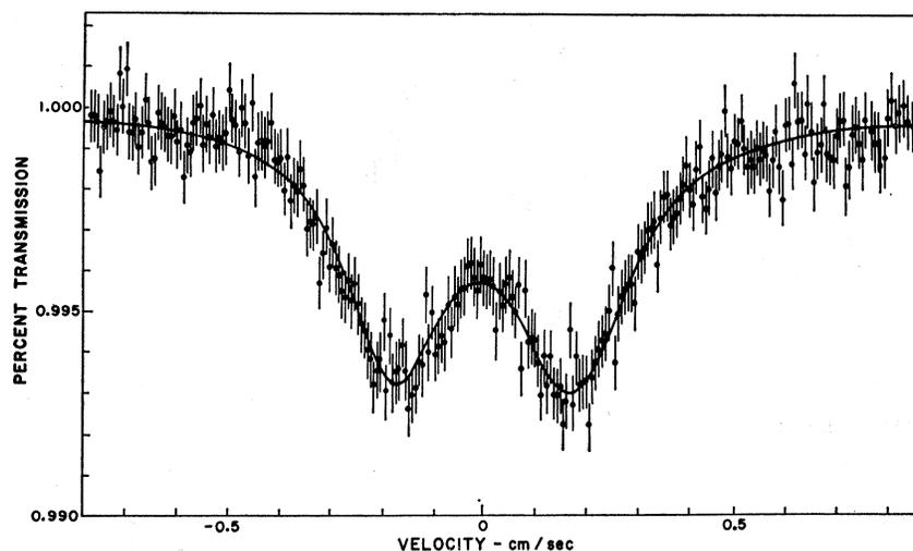
FIG. 5. Mössbauer absorption spectra for the 86.5-keV state of  $Gd^{155}$  at 4.2°K for a  $GdAl_2$  absorber containing 15 mg/cm<sup>2</sup> of  $Gd^{155}$ . These data have been corrected for nonresonant background.
