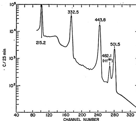
FIG. 2. Spectrum of  $\gamma$  rays from  $\text{Hf}^{180m}$  obtained with a Ge(Li) spectrometer.
