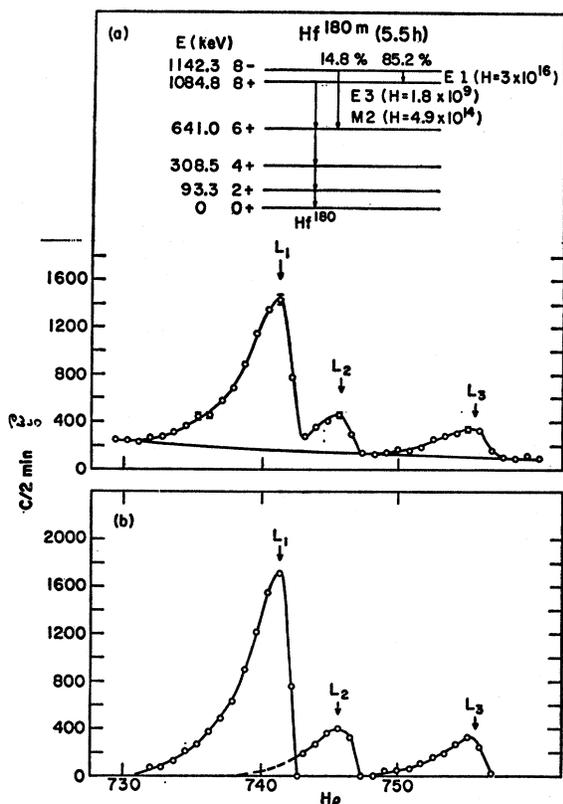
FIG. 1 (a) Spectrum of  $L$ -conversion-electron lines of 57.5-keV transition from  $\text{Hf}^{180m}$  before correction for background and decay. The spectrum was obtained with a double-focusing spectrometer. The insert shows the decay scheme of  $\text{Hf}^{180m}$ . (b) Average spectrum of 5 runs of the type shown in (a). Each run was individually corrected for background and decay.
