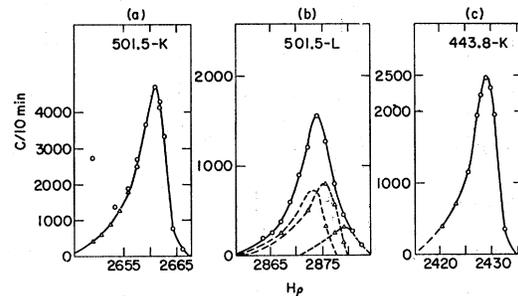
FIG. 4.  $K$ - and  $L$ -conversion electron lines of 501.5-keV transition in  $\text{Hf}^{180m}$  [(a) and (b)]. The two high points at the low-energy side of the 501.5-keV  $K$  line arise from the adjacent 443.8-keV  $L_{III}$  line. The  $K$  conversion line of the 443.8 transition (c) was used for intensity and energy calibration.
