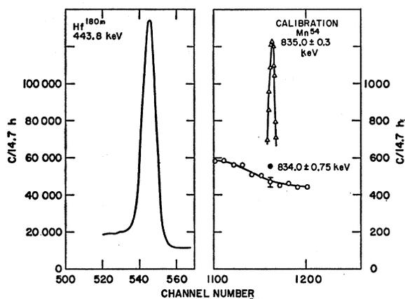
FIG. 5. The 834-keV region of the  $\text{Hf}^{180m}$   $\gamma$ -ray spectrum obtained with a Ge(Li) spectrometer is shown in juxtaposition with the 443.8-keV photopeak which was used for intensity calibration. The symbol  $\bullet$  indicates a hypothetical photopeak corresponding to an intensity ratio  $I_{834}/I_{443.8} = 5.7 \times 10^{-5}$ .
