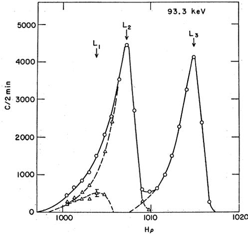
FIG. 3.  $L$ -conversion electron spectrum of 93.3-keV transition in  $\text{Hf}^{180m}$ . The line shapes were determined by linear extrapolation of a log-log plot.
