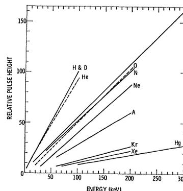
FIG. 7. Least-squares curves of relative pulse height from NaI(Tl) and CsI(Tl) versus particle energy for H and Kr for comparison.
