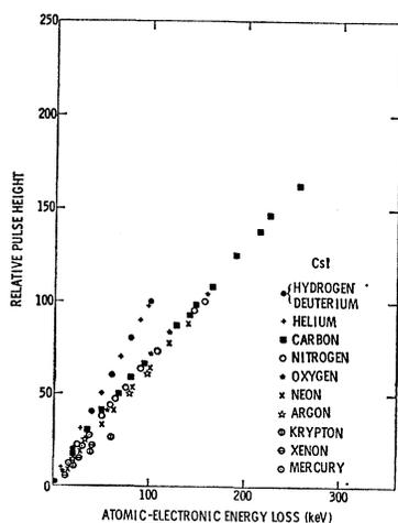
FIG. 12. Pulse height from CsI(Tl) versus calculated particle-energy-loss in atom-electron inelastic collisions. Two universal lines are defined.
