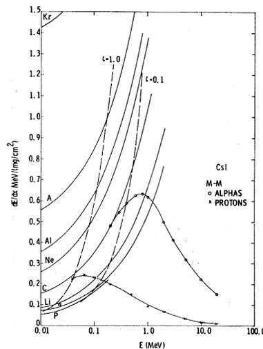
FIG. 10. Calculated stopping power of CsI versus incident particle initial energy. The Meyer-Murray curve for alpha particles and protons is shown for comparison.
