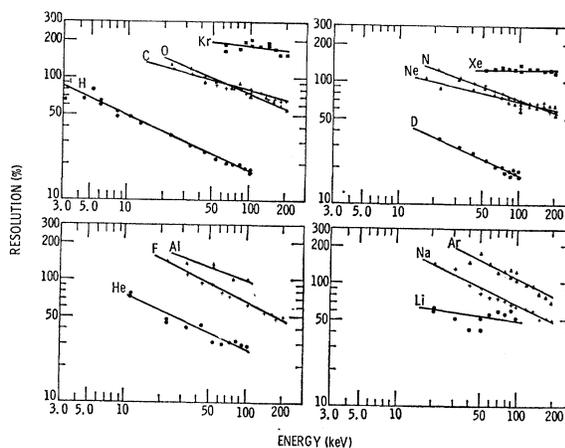
FIG. 3. Resolution of pulse-height distribution by NaI(Tl) versus particle energy for a number of heavy ions. Points are experimental. Curves are least-squares fits to the data.
