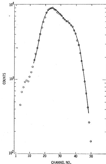
FIG. 8. Pulse height distribution from NaI(Tl) bombarded with 60 keV C<sup>+</sup> ions. Note the appearance of two pulse height distributions in coincidence.
