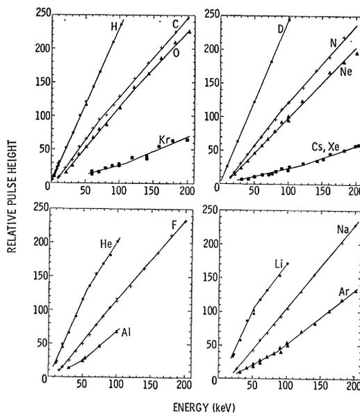
FIG. 2. Relative pulse height from NaI(Tl) versus particle energy for a number of heavy ions. Points are experimental. Curves are least-squares fits to the data.
