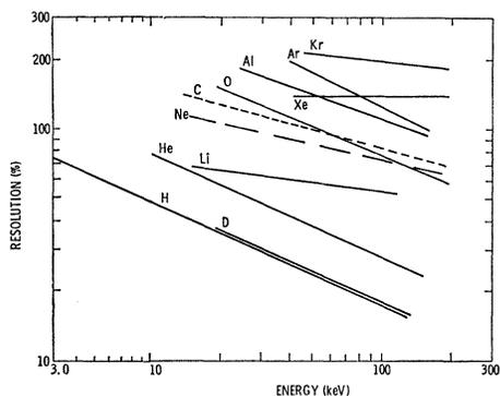
FIG. 5. Least-squares curves of resolution by NaI(Tl) versus particle energy. A composite of the separate curves.
