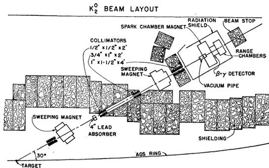
FIG. 1. Beam layout.
