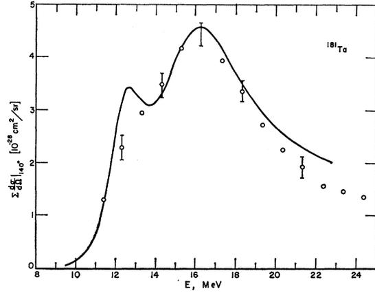
FIG. 23. Total quasi-elastic scattering cross section of  $^{181}\text{Ta}$  computed with the second set of parameters of Table IV. Experimental points as in Fig. 22 (energy scale is shifted up by 1.2 MeV).
