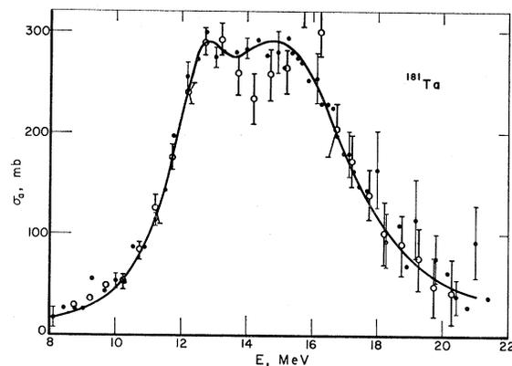
FIG. 20.  $\gamma$ -absorption cross section of  $^{181}\text{Ta}$  from Refs. 25 and 29. (Data from Ref. 29 is multiplied by 0.652.) The theoretical curve is computed with the first set of parameters of Table IV.
