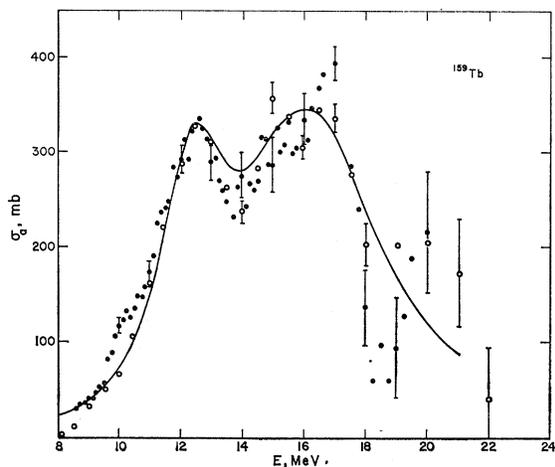
FIG. 17.  $\gamma$ -absorption cross section of  $^{159}\text{Tb}$  from Ref. 28 (circles, multiplied by 1.07) and from Ref. 29 (dots). The theoretical curve is computed with the second set of parameters of Table III.
