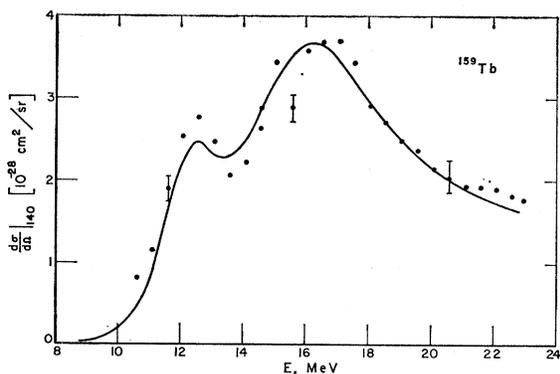
FIG. 18. Total quasi-elastic scattering cross section of  $^{159}\text{Tb}$  from Ref. 21 (multiplied by 0.823; energy scale is shifted up by 0.6 MeV). The theoretical curve is computed with the first set of parameters of Table III.
