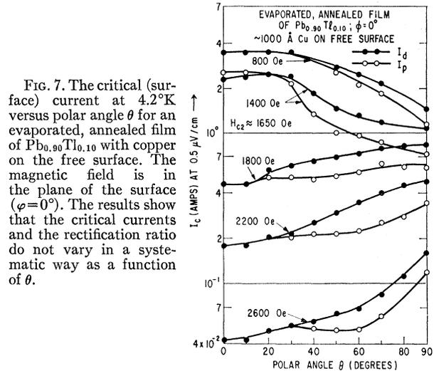
FIG. 7. The critical (surface) current at  $4.2^\circ\text{K}$  versus polar angle  $\theta$  for an evaporated, annealed film of  $\text{Pb}_{0.90}\text{Tl}_{0.10}$  with copper on the free surface. The magnetic field is in the plane of the surface ( $\phi = 0^\circ$ ). The results show that the critical currents and the rectification ratio do not vary in a systematic way as a function of  $\theta$ .
