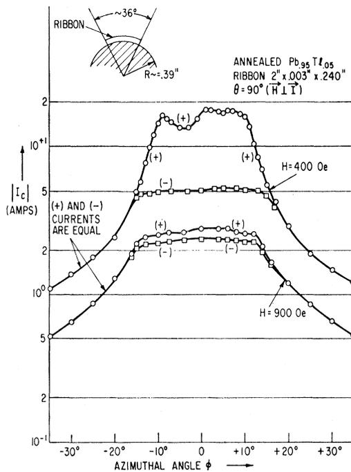
FIG. 12. The critical transport currents of opposite polarities for an annealed and curled  $\text{Pb}_{0.95}\text{Tl}_{0.05}$  ribbon at  $4.2^\circ\text{K}$  versus the angle that steady fields of 400 and 900 Oe make with the chord of the arc. The results demonstrate that partial rectification occurs when the magnetic field becomes tangent to some portion of the major surfaces and a perpendicular field distribution as shown in Fig. 10(c) is obtained.
