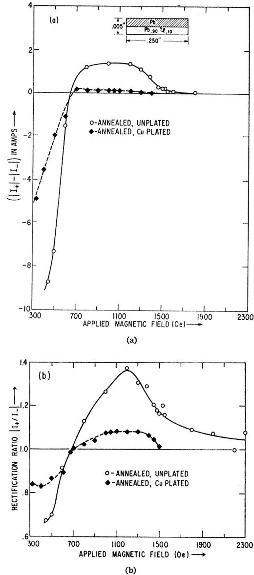
FIG. 3. The (a) absolute and (b) relative difference in the critical currents of opposite polarities of the sample of Fig. 2 before and after copper plating.
