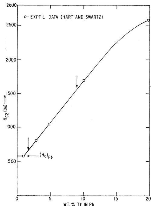
FIG. 4. A plot of  $H_{c2}$  at 4.2°K versus wt % Tl in Pb, taken from the experimental data of Hart and Swartz (Ref. 4).
