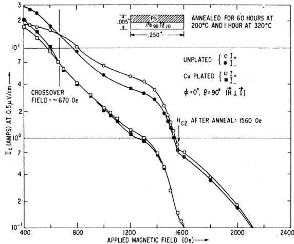
FIG. 2. The critical (surface) current at 4.2°K versus applied field for an annealed bimetallic strip of Pb-Pb<sub>0.90</sub>Tl<sub>0.10</sub>. The results show that the critical currents and the rectification are greatly diminished after copper plating.
