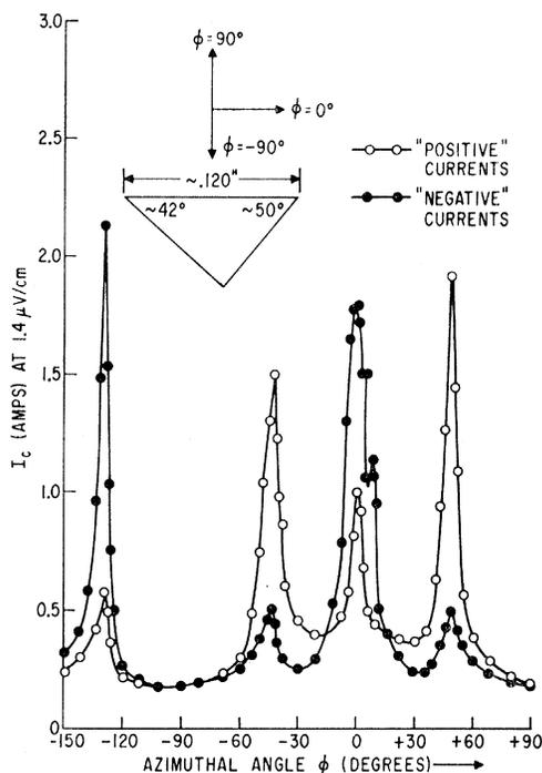
FIG. 14. Reproduced from Ref. 1. The critical current at  $4.2^\circ\text{K}$  of a well-annealed and polished prism of  $\text{Pb}_{0.95}\text{Tl}_{0.05}$  as a function of azimuthal angle  $\phi$  ( $\mathbf{H} \perp \mathbf{I}$ ) at a magnetic field of 700 Oe. The results show that the critical (surface) currents of opposite polarities go through maxima of significantly different magnitudes when the magnetic field vector is aligned parallel to a surface.
