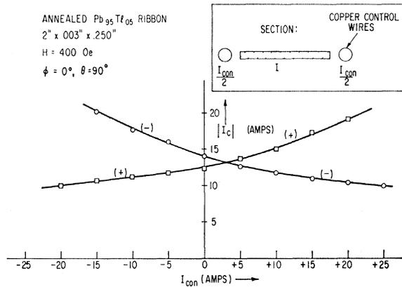
FIG. 11. The critical transport currents of opposite polarities in an annealed  $Pb_{0.95}Tl_{0.05}$  ribbon versus the current in the control wires. The results show that partial rectification occurs in the presence of a perpendicular field distributed as shown in Fig. 10(c).
