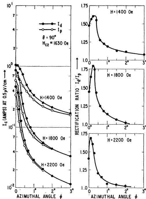
FIG. 6. The critical (surface) currents and rectification ratio at  $4.2^\circ\text{K}$  as a function of azimuthal angle  $\phi$  for the sample of Fig. 5. The results show that the rectification ratio approaches unity as the perpendicular component of the magnetic field ( $\propto \phi$ ) is increased.
