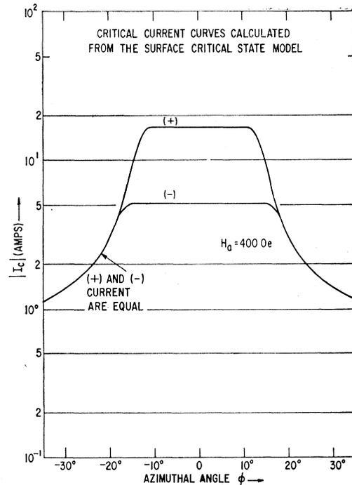
FIG. 13. Critical current curves calculated from the critical state model [Eq. (2)] for the geometric arrangement of Fig. 12 and the assumption that  $J_c(H_\perp) = J_0 / (1 + |H_\perp / H_{L,1/2}|)$  where  $J_0$  and  $H_{L,1/2}$  are taken to be 85 A/cm (for the two surfaces combined) and 4.8 Oe, respectively.
