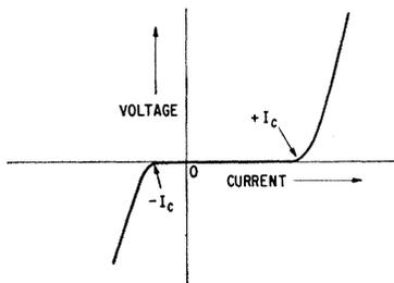
FIG. 1. A schematic of an asymmetric current-voltage characteristic. We denote this property as "partial rectification."
