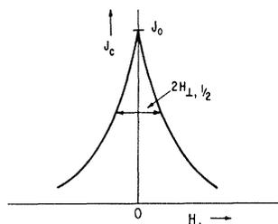
FIG. 8. A schematic of the microscopic critical surface current as a function of the local perpendicular magnetic field, as assumed in the present model.
