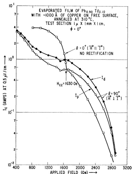
FIG. 5. The critical (surface) current at 4.2°K versus applied field of an evaporated, annealed film of  $Pb_{0.90}Tl_{0.10}$  with a flash of copper on the free surface. When the magnetic field is parallel to the surfaces and perpendicular to the current direction, partial rectification is observed; when the magnetic field and current directions are coincident, no rectification is observed.
