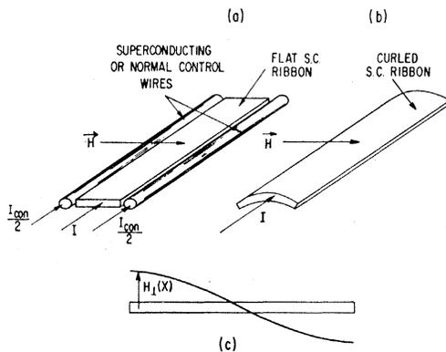
FIG. 10. A schematic showing experimental techniques for achieving a distribution of the perpendicular field as shown in (c).
