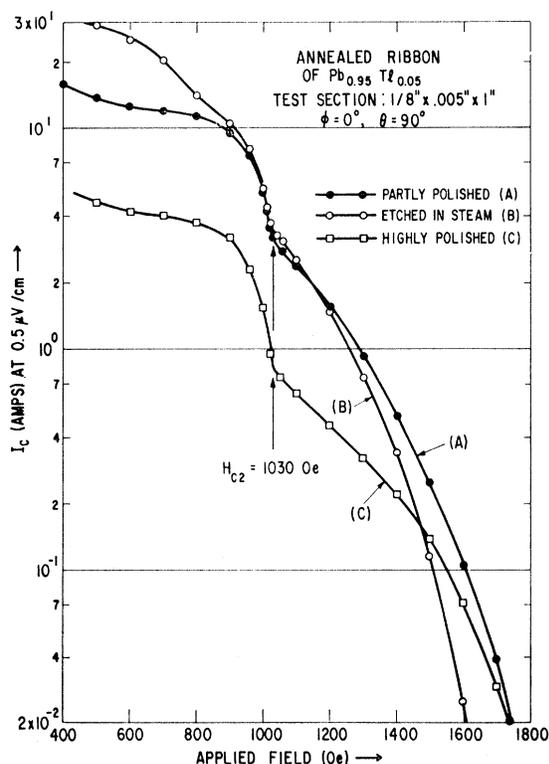
FIG. 2. The critical surface current at  $4.2^\circ\text{K}$  versus magnetic field for an annealed  $\text{Pb}_{0.95}\text{Tl}_{0.05}$  ribbon ( $\varphi=0^\circ$ ,  $\theta=90^\circ$ ) after successive surface preparations. The results show that, except near  $H_{c2}$ , the highly polished sample carries the least current.
