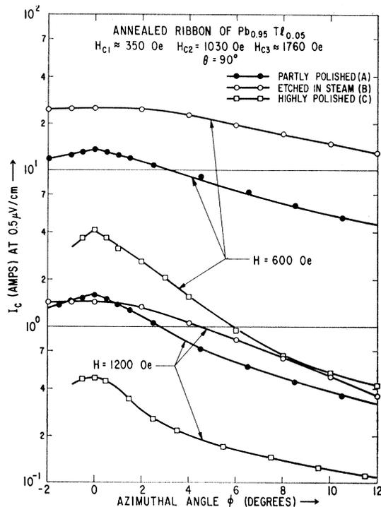
FIG. 3. The critical surface current at  $4.2^\circ\text{K}$  of an annealed  $\text{Pb}_{0.95}\text{Tl}_{0.05}$  ribbon as a function of azimuthal angle  $\varphi$ . The results show that the highly polished sample is the most sensitive and the etched sample the least sensitive to the perpendicular component of the applied magnetic field.
