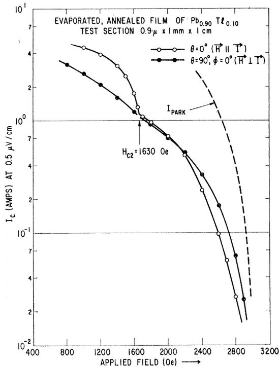
FIG. 4. The critical surface current at 4.2°K versus magnetic field for an evaporated and annealed film of  $\text{Pb}_{0.90}\text{Tl}_{0.10}$ . Below  $H_{c2}$  the critical current is larger when the field and current are parallel; above  $H_{c2}$ , when perpendicular. In both cases the critical surface current is much less than the calculated value (Ref. 12) (as shown).
