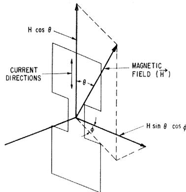
FIG. 1. The definition of the polar angle  $\theta$  and the azimuthal angle  $\phi$  in terms of the current  $I$ , the field  $H$ , and the sample geometry.
