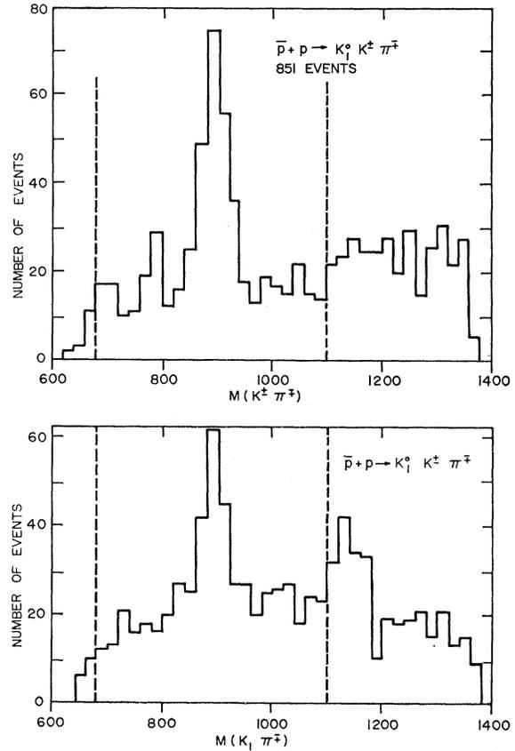
FIG. 9. Effective mass of neutral and charged  $(K\pi)$  combinations from the reaction  $\bar{p}+p \rightarrow K_1K^\pm\pi^\mp$ . The region between the dashed lines was used in fitting for the  $K^*$  mass difference.
