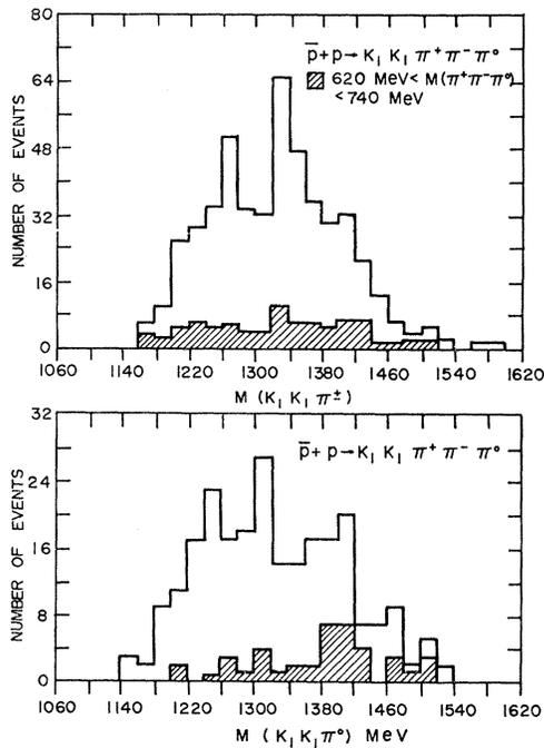
FIG. 7. Combined mass of  $(K_1K_1\pi^0)$  and  $(K_1K_1\pi^\pm)$  from the reaction  $\bar{p}+p \rightarrow K_1K_1\pi^+\pi^-\pi^0$ . The shaded region indicates events where the  $(\pi^+\pi^-\pi^0)$  combined mass is between 620 and 740 MeV.
