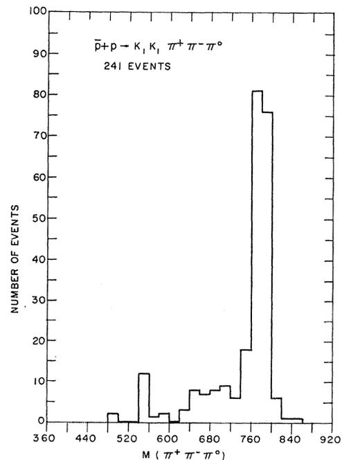
FIG. 2. Combined mass of  $(\pi^+\pi^-\pi^0)$  from the reaction  $\bar{p}+p \rightarrow K_1 K_1 \pi^+\pi^-\pi^0$ .
