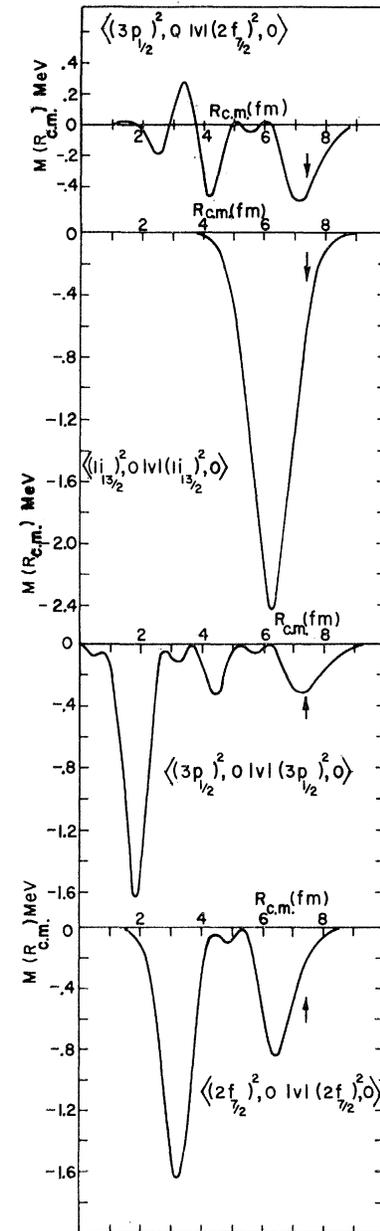
FIG. 4.  $M(R_{c.m.})$ , as defined in Eq. (31) for the  $I=0$  states of various configurations near the Fermi surface of  $\text{Pb}^{208}$ . The arrows indicate the location of the nuclear radius.
