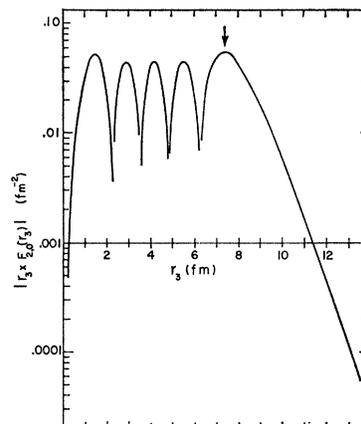
FIG. 2. Form factor for the reaction  $\text{Pb}^{208}(p,t)\text{Pb}^{206}$  leading to the 0.8-MeV  $2^+$  state in  $\text{Pb}^{206}$ . The mean-square radius of the triton is taken to be  $(1.7 \text{ F})^2$ . The arrow indicates the location of the nuclear radius.
