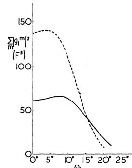
FIG. 3. The nuclear matrix element for noncoplanar scattering calculated using distorted waves. The target is  $\text{Li}^6$ , the incident energy is 185 MeV, and the optical potential parameters are taken from Ref. 9. The scattering angle  $\theta_L$  is  $35.5^\circ$ . For the full line the length parameter is the same as in Fig. 2, while for the dashed line the length parameter has been increased to 2.24 F.
