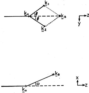
FIG. 1. The scattering system. (In the laboratory system, the scattering angle and the angle of noncoplanarity are represented by the symbols  $\theta_L$  and  $\omega_L$ .)
