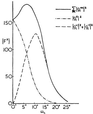
FIG. 2. The components of the nuclear matrix element for noncoplanar scattering calculated using plane waves. The dashed lines show the components for  $m=0$  and  $m=\pm 1$  and the full line is the sum of these. The parameters are those of set B in Table I, the target is  $\text{Li}^6$ , and the incident energy is 185 MeV. The scattering angle  $\theta_L$  is  $35.5^\circ$ .
