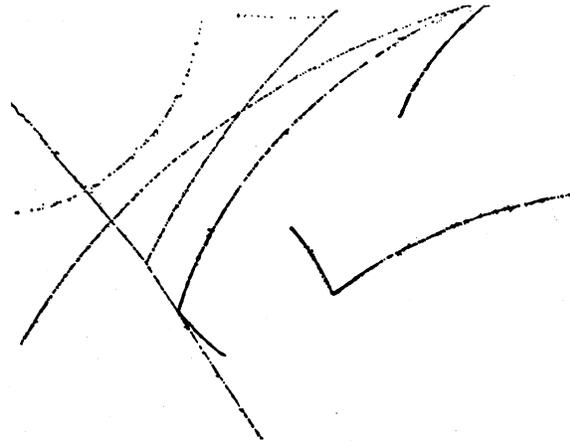
Fig. 1. A typical  $\pi^+ + d \rightarrow p + p$  event as seen in the bubble chamber. The pion enters from upper right. Pions which did not interact are also seen. They stop in the chamber and decay  $\pi^+ \rightarrow \mu^+ \rightarrow e^+$ .
