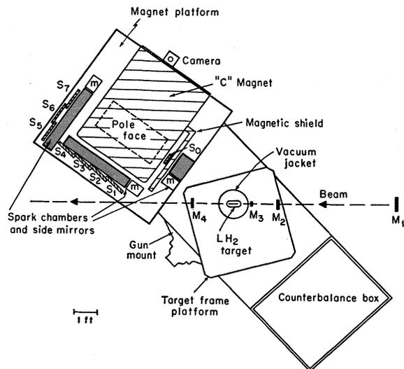
FIG. 3. Diagram of experimental area, showing spectrometer and monitor system. The beam-monitor counters ( $M_1, M_2, M_3, M_4$ ) are not shown to scale. The letter  $m$  refers to side mirrors on the spark chambers, and  $S_i$  are the spectrometer counters.
