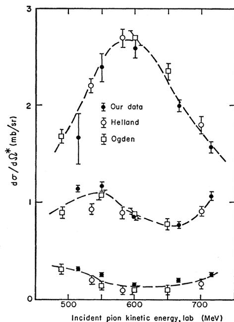
FIG. 14. The  $\pi^-p$  differential cross sections at proton angles of 60 deg (top), 18 deg (center), and 37 deg (bottom) as a function of beam energy. The dashed line is intended only to guide the eye.
