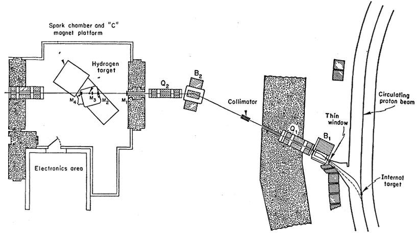
in Fig. 2. This beam, whose properties are given in Table I, was focused on a cylindrical liquid-hydrogen target of 3.75-in. diam and 5.77-in. effective length. The beam was monitored by the  $M_1$ ,  $M_2$ , and  $M_3$  scintillation counters in front of the target and  $M_4$  behind the target in anticoincidence.
