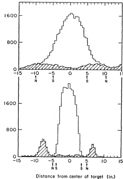
FIG. 6. Two histograms of the calculated point of interaction in the target (see text). The top is for the spectrometer set at 18 deg, the bottom at 60 deg. "N" and "S" refer to the cutoffs used for normalization and spectra, respectively. The shaded areas refer to the empty-target (i.e., background) spectrum.
