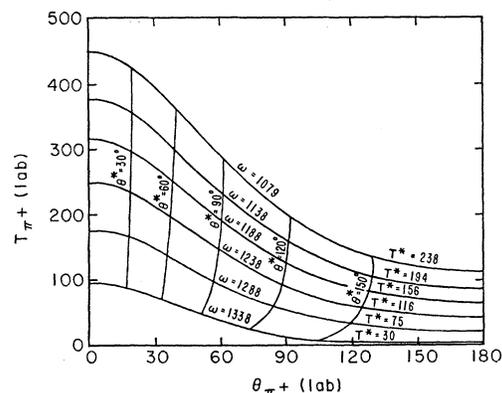
FIG. 1. Pion kinematics for  $\pi^-p \rightarrow \pi^+\pi^-n$  at an incident energy of 599 MeV. The solid lines represent lines of constant c.m.  $\pi^+$  angle ( $\theta^*$ ) and  $\pi^-n$  recoil mass ( $\omega$ ) [equivalent to c.m. kinetic energy of the  $\pi^+$  ( $T^*$ )] as labeled.  $T_{\pi^+}$  (lab) refers to the laboratory kinetic energy of the  $\pi^+$  (in MeV); and  $\theta_{\pi^+}$  (lab) is the lab angle of the  $\pi^+$  in degrees.
