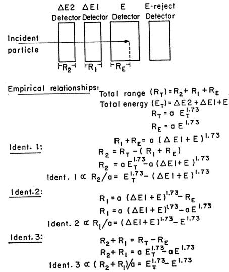
FIG. 3. A schematic derivation of the three identification pulses generated by the three-counter particle identifier.
