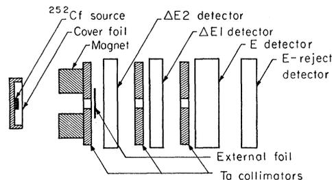
FIG. 1. Experimental arrangement of the  $^{252}\text{Cf}$  source with respect to the cover foil, magnet, external foil, collimators and detectors.
