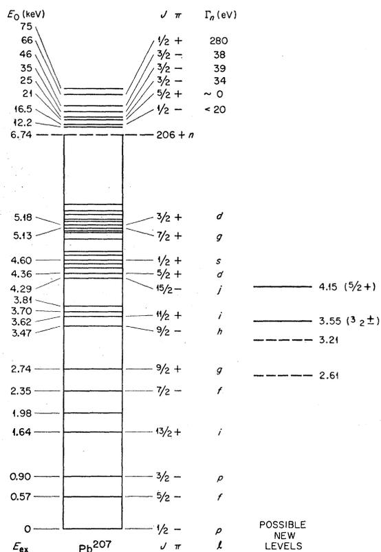
FIG. 5. Energy levels in  $^{207}\text{Pb}$ . Levels observed up to 75 keV above the neutron separation energy are given with neutron widths and probable spin assignments. Two previously unobserved states between 2.61 and 4.1 MeV, discovered in the capture gamma-ray spectra, are shown on the right. Uncertainty as to the order of the transition makes it impossible to identify which of the two possible locations for each level is the correct one.
