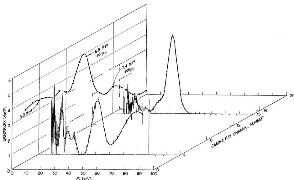
Yield of Gamma Rays as a Function of Neutron Energy for  $^{207}\text{Pb}$  Target (Gamma Rays in 20 Channel, Neutrons in-128 Channel).
