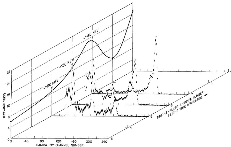
Yield of Gamma Rays as a Function of Neutron Energy for  $^{207}\text{Pb}$  Target (Neutrons in 8 Channel, Gamma Rays in 256 Channel).
