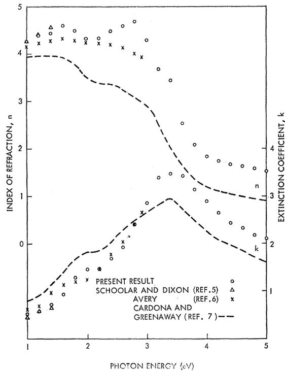
FIG. 6. The optical constants of PbS obtained by previous investigators compared with the present results.
