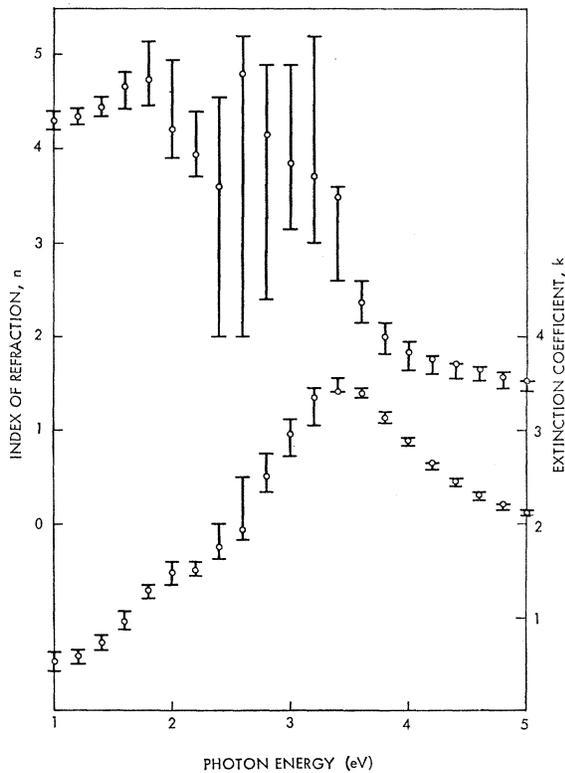
FIG. 5. The index of refraction  $n$  and extinction coefficient  $k$  obtained from the data for the 490-Å film.
