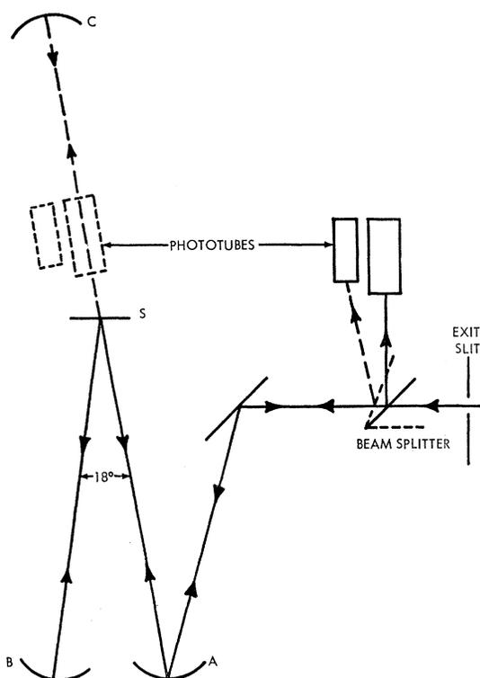
FIG. 1. Schematic of the optical system. The position of the photomultiplier tubes is shown for reflectance (solid outline) and transmittance (broken outline) measurements. The sample position is denoted by S and the positions of the identical spherical mirrors by A, B, and C.
