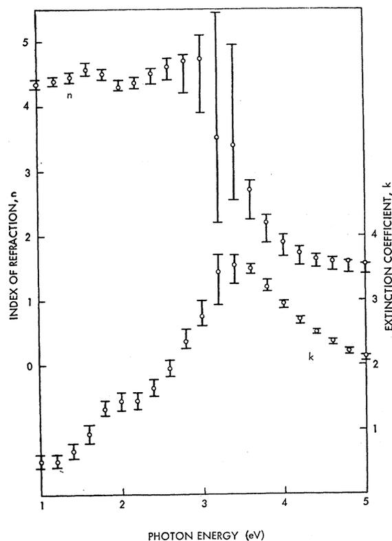
FIG. 4. The index of refraction  $n$  and extinction coefficient  $k$  obtained from the data for the 260-Å film.
