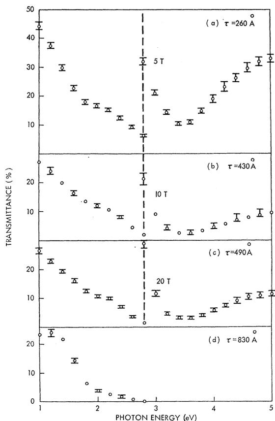
FIG. 3. Transmittance data. The transmittance data are shown in the same manner as the reflectance data in Fig. 2, except for a scale change at 2.8 eV. From 2.8 to 5.0 eV, the points plotted are 5*T*, 10*T*, and 20*T* for the 260-, 430-, and 490-Å films, respectively.
