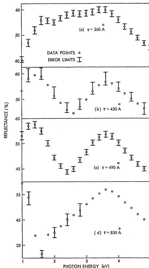
FIG. 2. Reflectance data. At each point for which the optical constants were calculated, limit marks are used to show the maximum error in the data.
